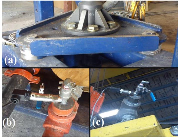
**Figure 4.36:** (a) load cells, (b) upstream pressure sensor and (c) downstream pressure sensor used in testing frame in Advanced Drilling Laboratory at MUN.
