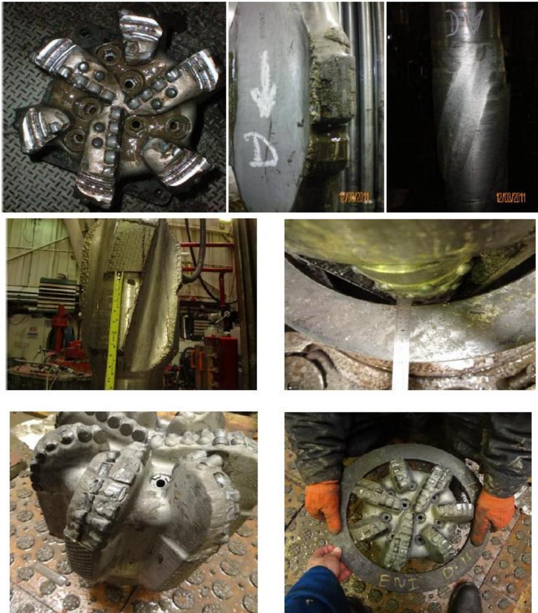
**Figure 2.13:** Photos of damaged and worn out drill bits, stabilizers (Wright *et al.*, 2014).
