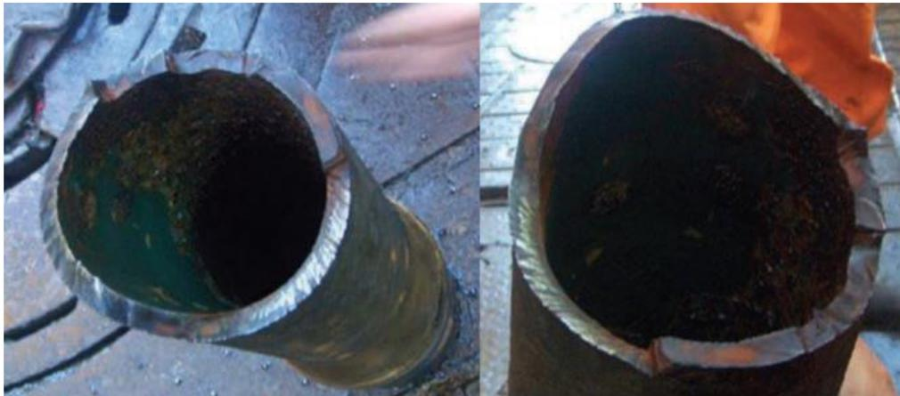
**Figure 2.10:** Fracture of the drillpipe twistoff (Raap *et al.*, 2012).
