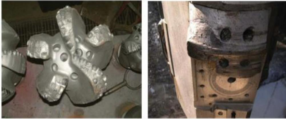
**Figure 2.9:** Photo of drill bit and tool failures (Akinniranye *et al.*, 2009)
