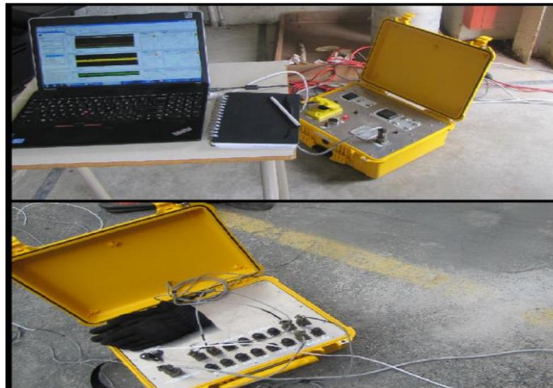
**Figure 4.37:** Mobile DAQ system in Advanced Drilling Laboratory at MUN.
