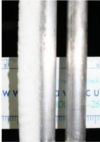
Figure 2.2 Ice accretion on parallel cylindrical probes.
