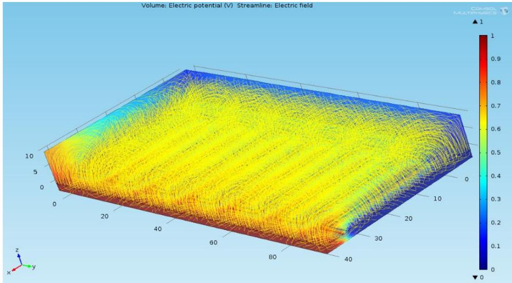
Figure 4.12 Sensitivity Analysis showing fringing field lines
