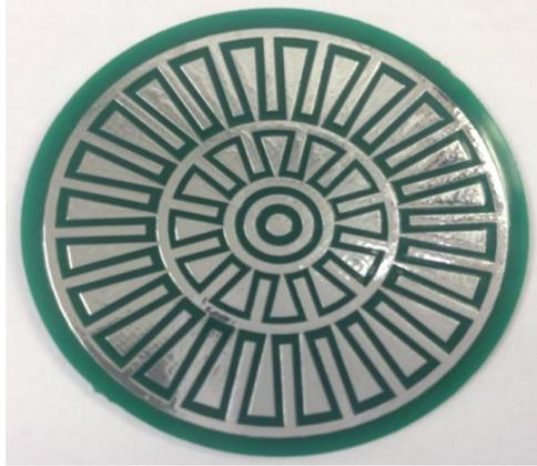
Figure 4.21 Fabricated prototype 3 Sensor Plate
