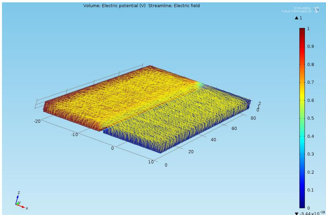
Figure 8.3 Field lines passing through water and ice
