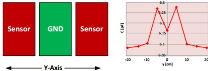
Figure 4.3 Central Ground Symmetry.
