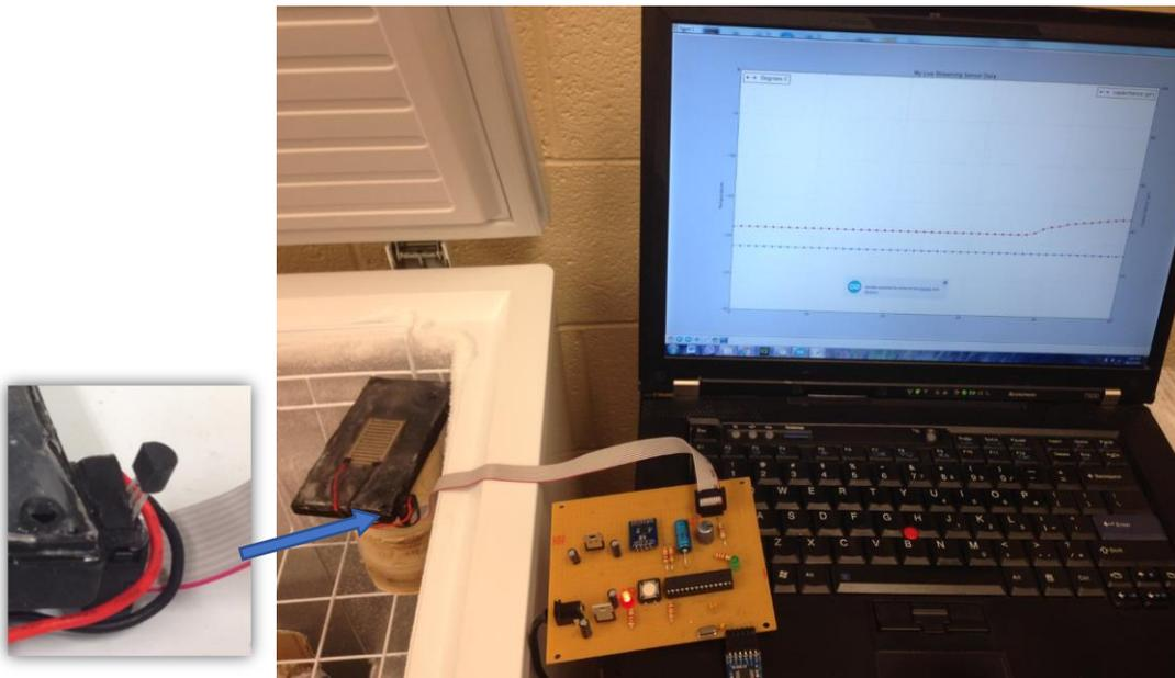
Figure 7.1 Experimental Setup showing the temperature sensor
