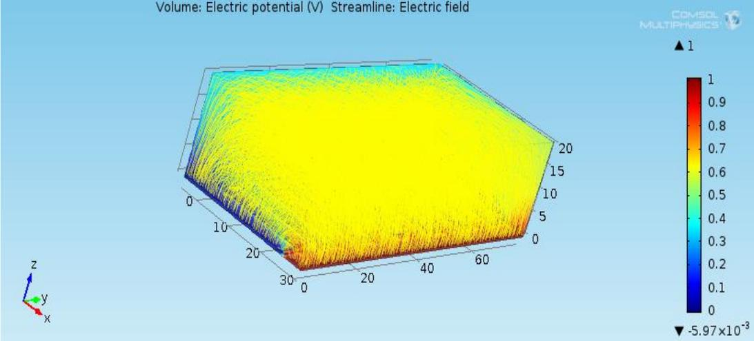
Figure 4.18 Sensitivity Analysis showing fringing field lines
