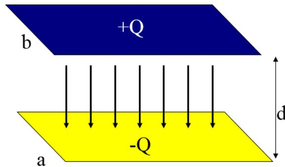
Figure 3.2 Configuration of a parallel plate capacitor
