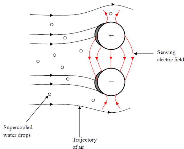
Figure 2.1 Super cooled droplets approaching a capacitive probe
