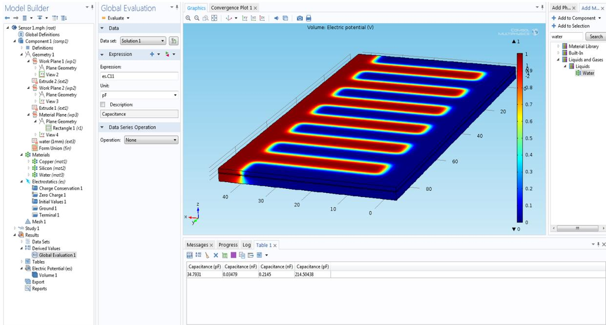
Figure 4.8 COMSOL simulation of sensor tracing with 1mm water film
