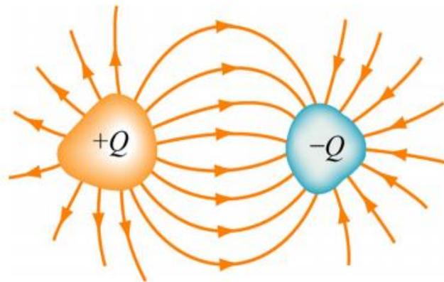
Figure 3.1 Basic configuration of a capacitor
