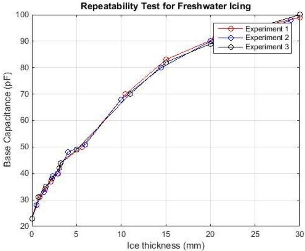
Figure 7.5 Results of 3 Experiments using fresh water
