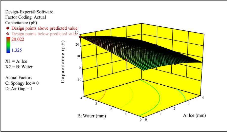
Figure 8.6 3D Capacitance plot for 1mm air gap and 0mm Spongy ice.
