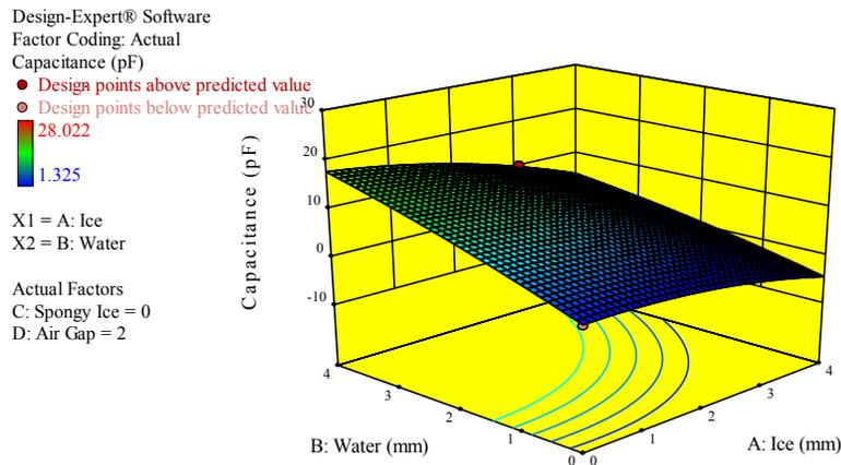
Figure 8.8 3D capacitance plot for 2mm air gap spongy ice 0mm
