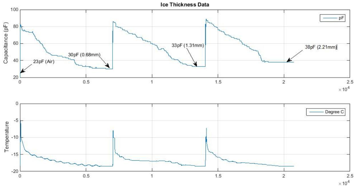
Figure 7.8 Data processing output for ice accretion experiment using Sea water
