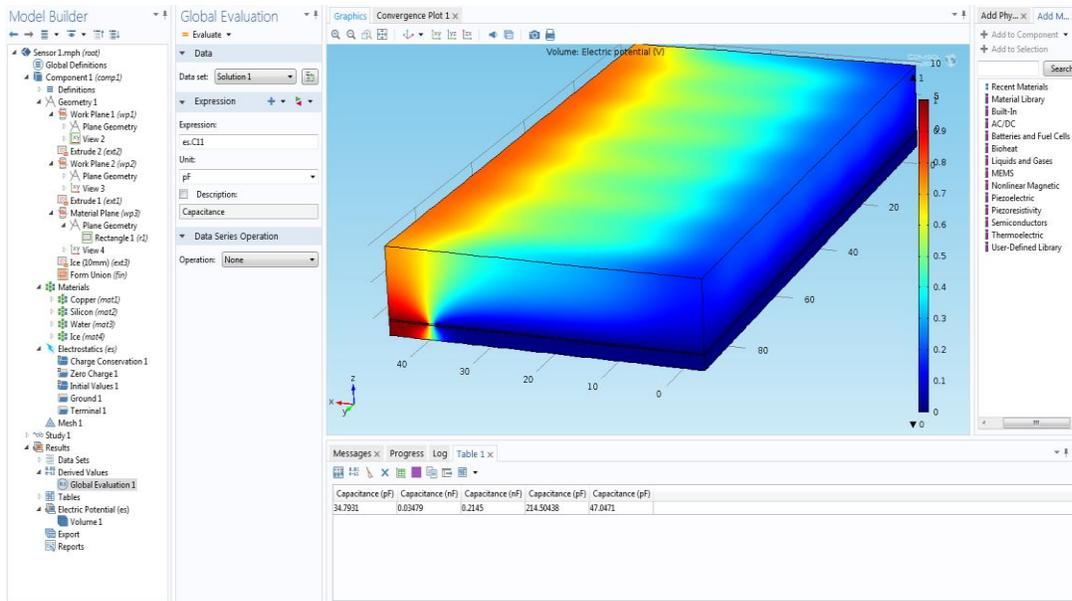
Figure 4.9 COMSOL Simulation for change in capacitance due to 10mm icing
