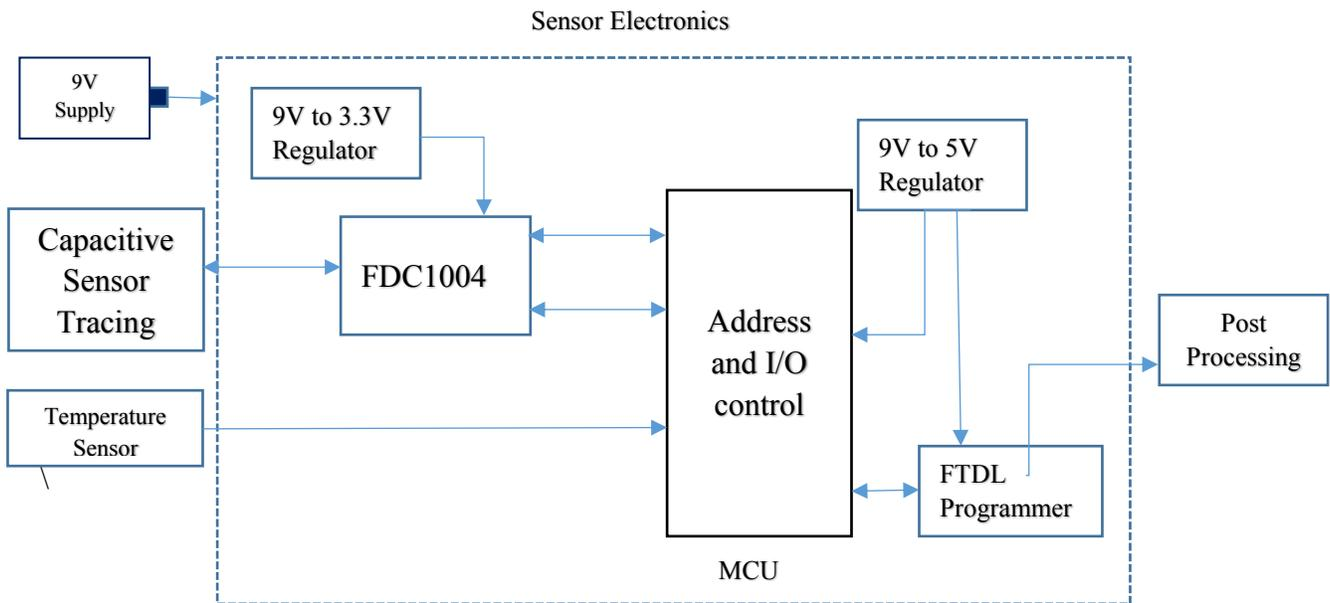
Figure 5.1 Block diagram showing sensor electronics
