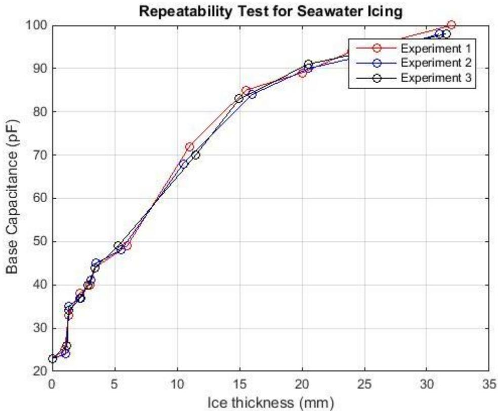
Figure 7.9 Results of 3 Experiments using Seawater (35PSU at Room temperature)
