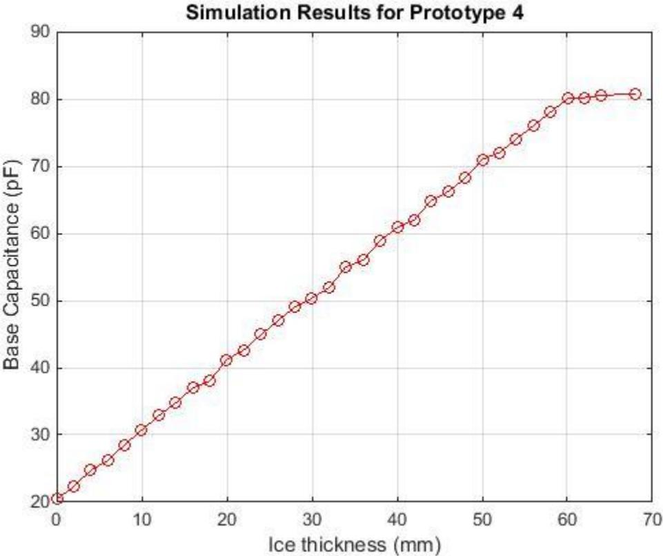
Figure 4.23 Simulation results for capacitance vs Ice thickness for prototype 4
