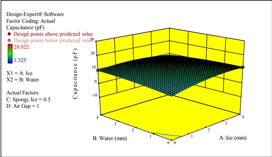
Figure 8.7 3D Capacitance plot for 1 mm air gap 0.5mm spongy ice
