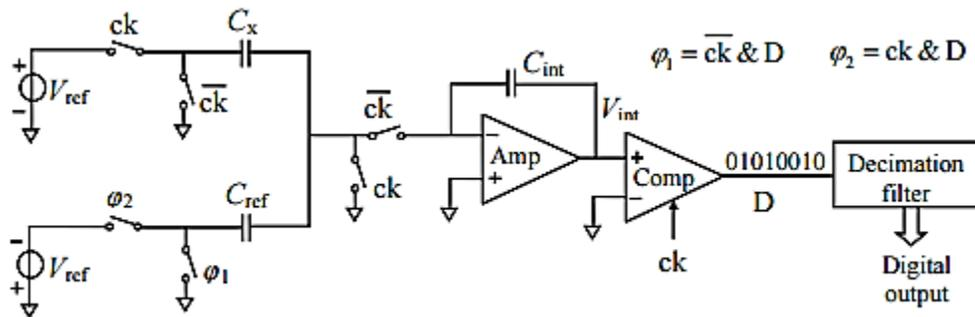
Figure 5.2 Capacitance to Digital Conversion using Sigma-delta
