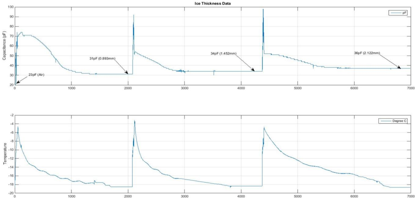
Figure 7.3 Data processing output for ice accretion experiment using fresh water
