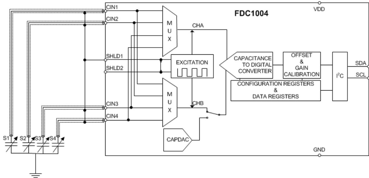
Figure 6.3 Single-Ended Configuration with CAPDAC enabled
