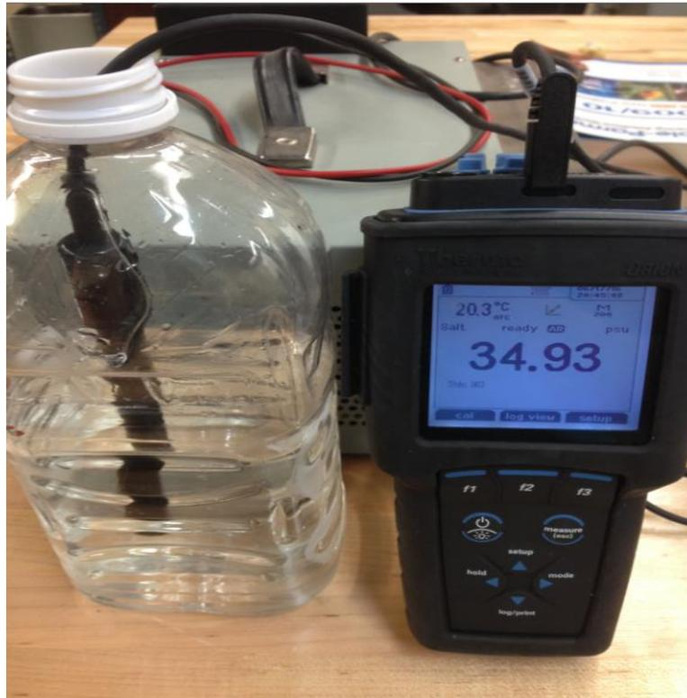
Figure 7.7 Laboratory preparation of sea water at 20.3°C
