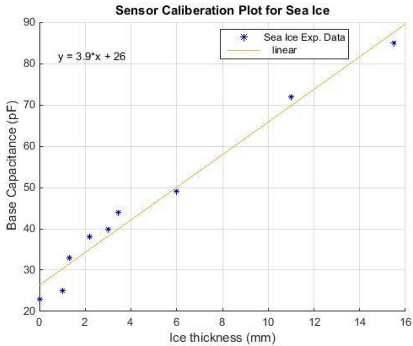
Figure 7.12 Sensor Calibration Plot for seawater
