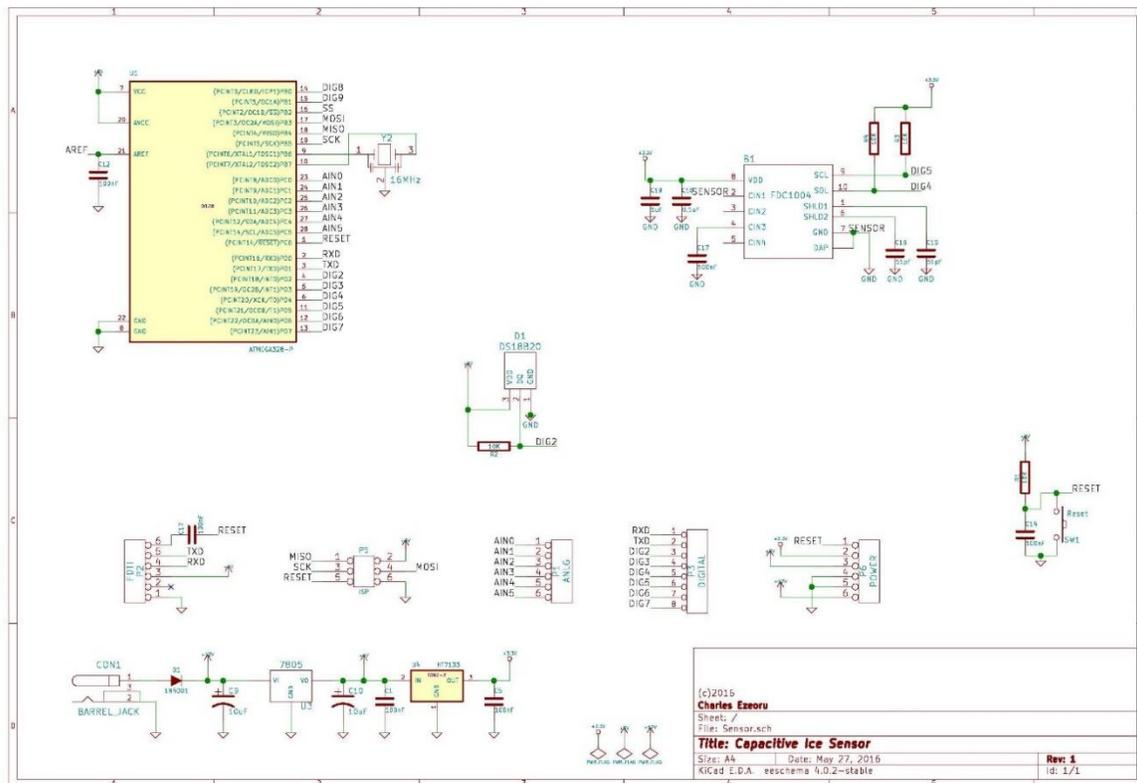
Figure 6.2 Overall system Schematic
