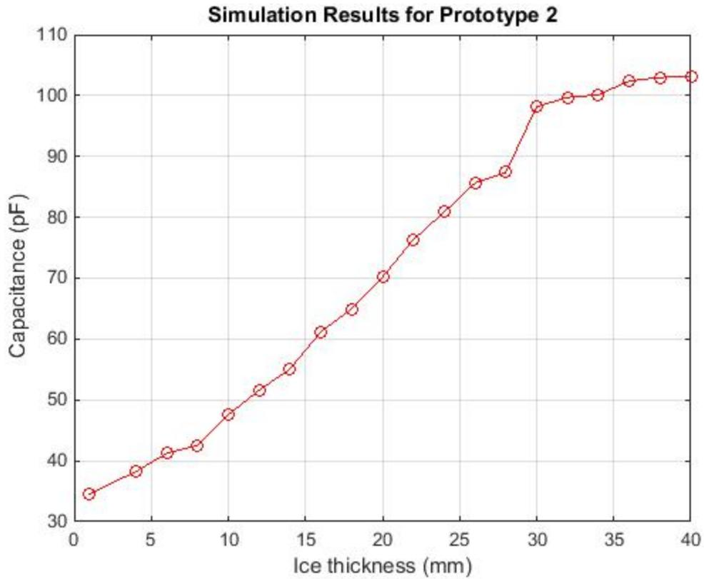
Figure 4.11 Simulation results for capacitance vs Ice thickness for prototype 2
