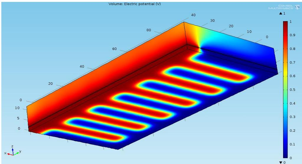
Figure 4.10 Bottom view of the electric field effect through silicon substrate
