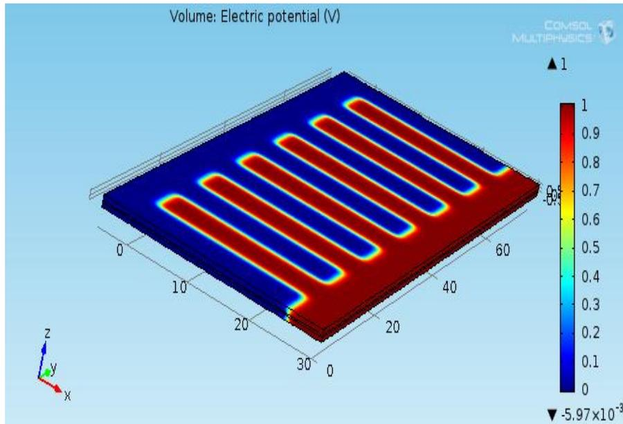
Figure 4.15 COMSOL simulation of sensor tracing with 1mm water film
