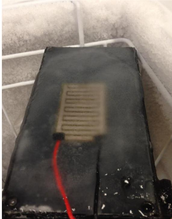
Figure 7.2 Ice thickness using fresh water (2.1mm)
