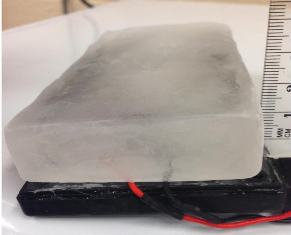
Figure 7.4 Experimental setup using ice slabs (20.5mm)
