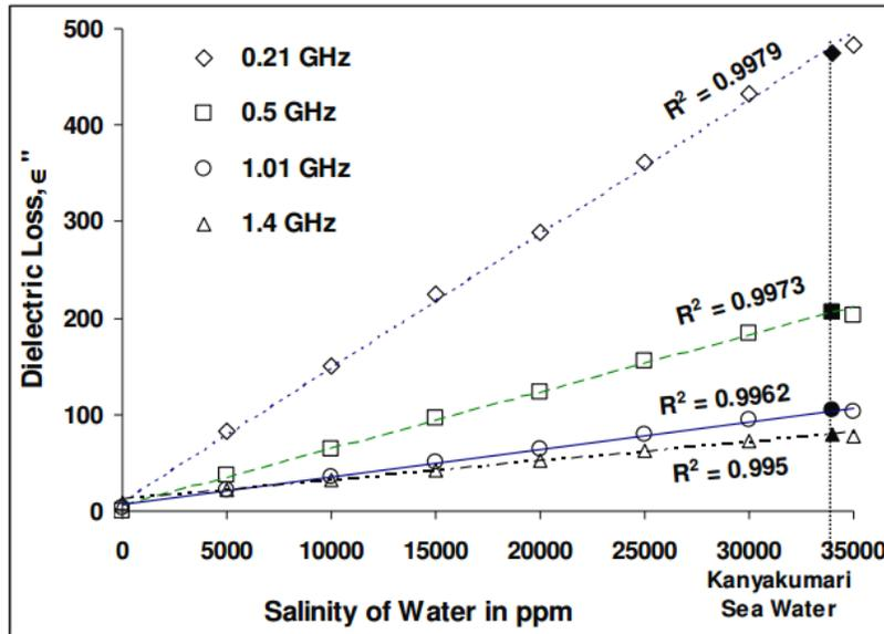
Figure 7.10 Variation of dielectric loss with Salinity
