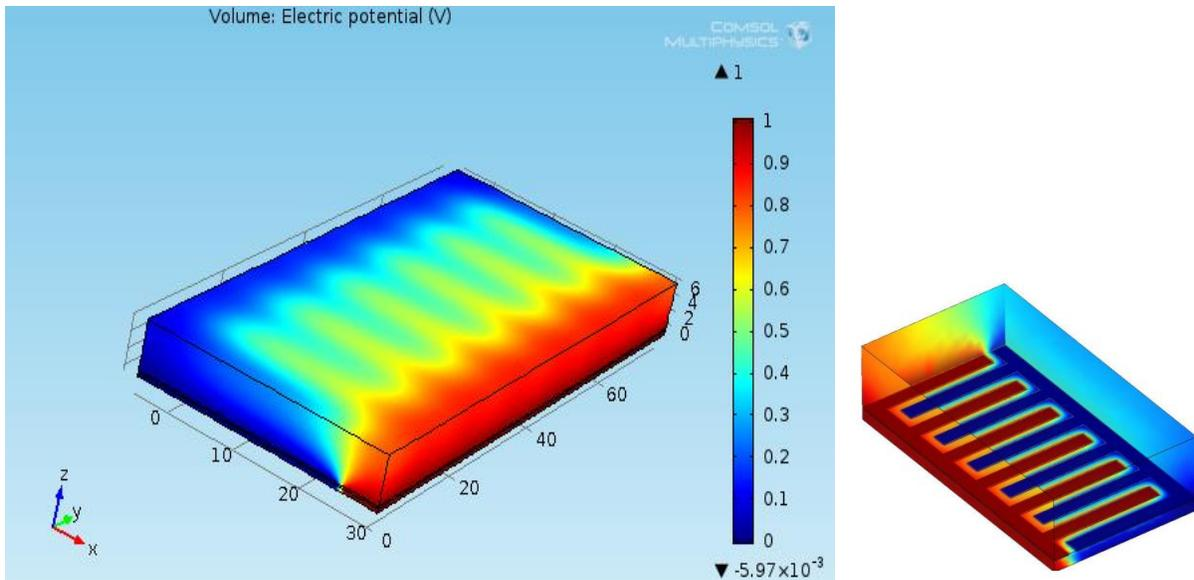
Figure 4.16 COMSOL Simulation for change in capacitance due to 10mm icing
