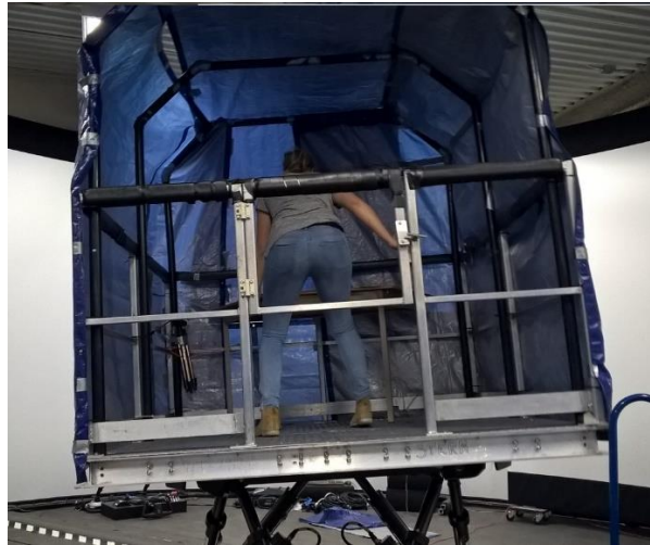
Figure 3.1: Picture showing the motion simulator and setup used for the study. A table is in front of the participant while he or she remains facing forward, unable to see outside of the simulator as a result of the cover.
