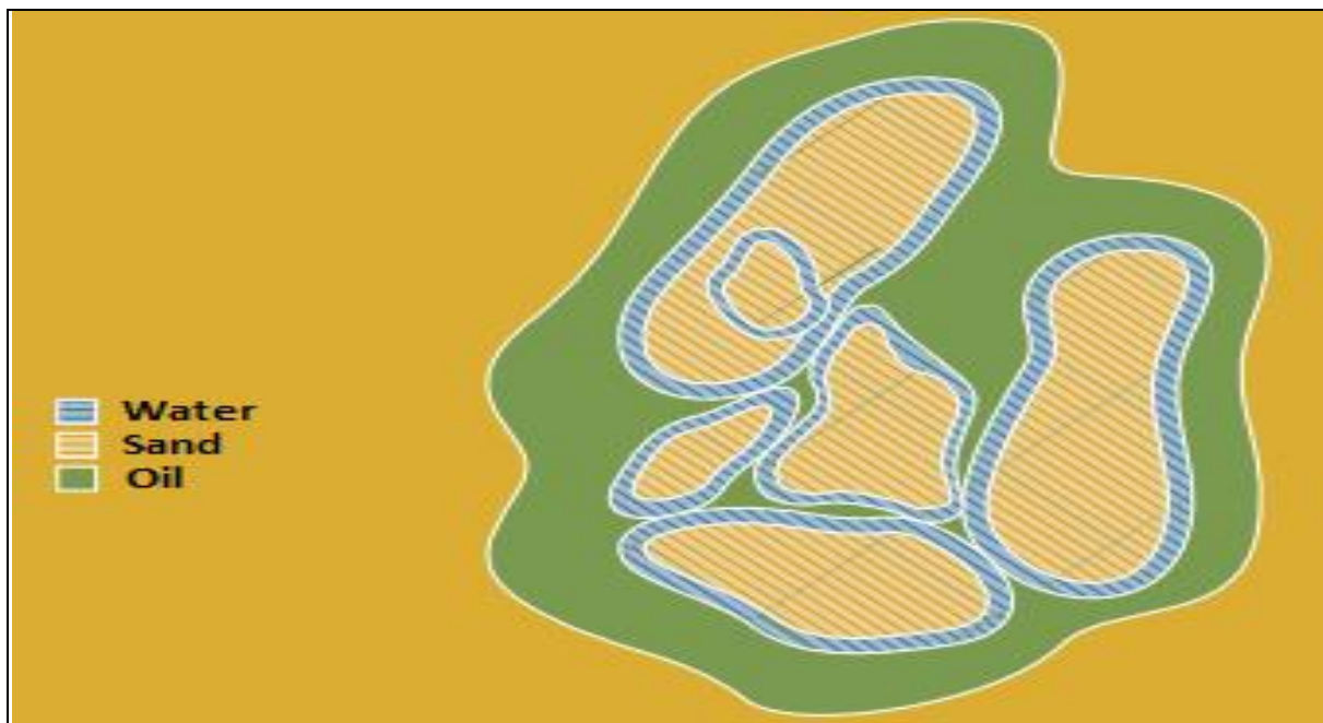
Figure 2: A Schematic View of an Oil Sand Particle in Alberta
