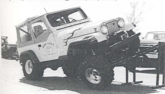
FIG: 3.7 Charlie Copsey tests his wheel travel on a specially-constructed ramp. Notice that all tires remain in contact with the ground, providing traction for the Jeep's four corners. (More on "ramping" in chapter four.)
