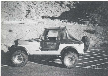
FIG: 4.33 Notice the sidewall tread protecting the sides of Victor's tires. This keeps rocks from slashing them. (Courtesy Victor Mokler)
