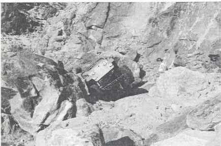
FIG: 3.12 On Sledgehammer trail, Jim shows that even 4x4s with lots of suspension travel sometimes “lift” tires. Lockers in both axles help him pull through this situation with no problems (Courtesy Jim Cole)
