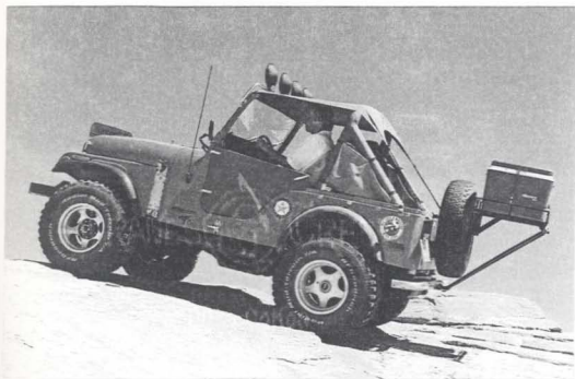
FIG: 4.31 The custom body lift blocks are visible between the body and the bumper at the back of Chip's Jeep.
