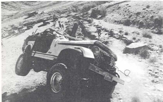
FIG: 4.12 As can be seen here, the roll bar has not folded over; but there is no cage kit to protect the front of the Jeep's cab section. The windshield has folded-in towards the driver. (Courtesy Mark Milner)
