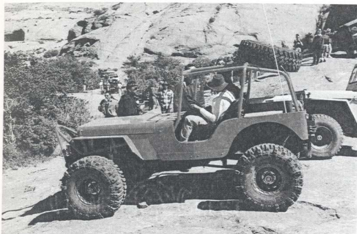
FIG: 3.17 This bright-pink Jeep boasts a hand-built body and custom-fabricated extended-travel suspension.
