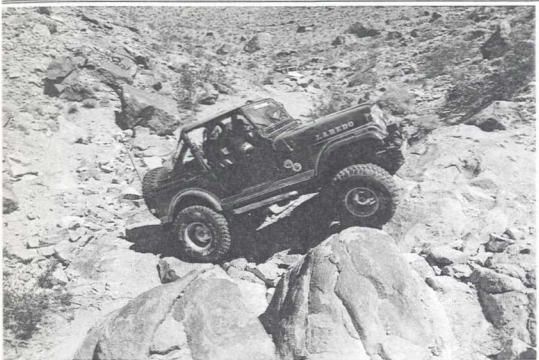
FIG: 4.14 Nerf bars under the body protect the rocker panels of the Neilsen's Jeep. (Courtesy Jim Broadbent)
