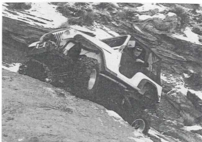
FIG: C.4 Jeff Beach shows what a competently built rig can do by climbing a near-vertical boulder. Notice the wheel travel on the rear axle. (Courtesy Jeff Beach)
