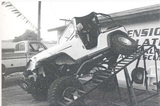
FIG: 3.6 Jeff Beach's Jeep—shown here backing up a ramp—has extensive wheel travel. Such vast travel helps to keep the Jeep's tires in contact with the rugged terrain. (Courtesy Jeff Beach)
