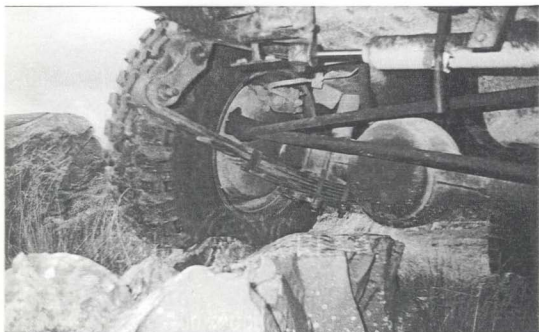
FIG: 5.4 An aired down tire conforms to the shape of the terrain, providing increased traction.
