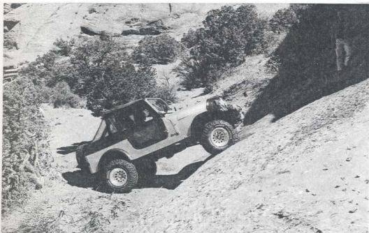
FIG: 4.34 Gearing and a locker combine to help Victor scale Tip-Over Challenge on Hell's Revenge trail. Chris Stephens, the trail leader, spots for Victor in the upper left corner. (Courtesy Victor Mokler)
