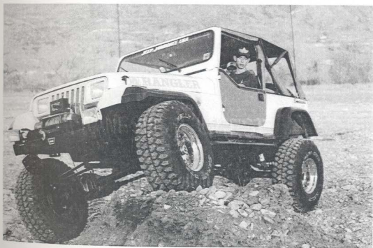
FIG: 4.20 Justin shows off the Wrangler's extensive front wheel travel. Notice the winch and nerf bars.
