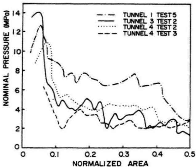
Figure A.1 Measured Pressure-Area Relationships (Master son et al., 1992).
