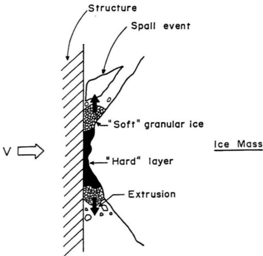
Figure A.2 Schematic of a High Pressure Zone.
