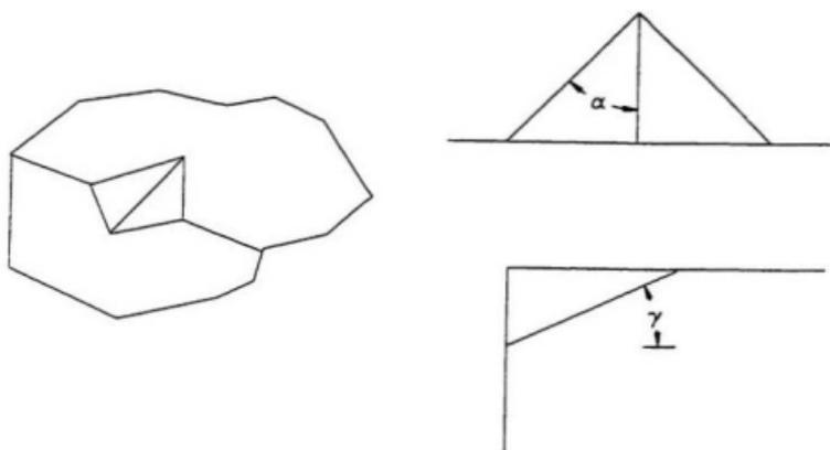
**Figure A.5 Definition of Penetration Geometry for a Wedge-Shaped Bow.**
