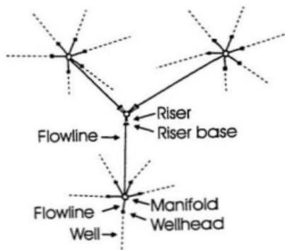
Figure 4.2 Configuration of subsea system
