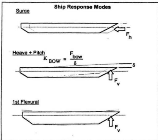
Figure A.4 Description of the Ice-Vessel Interaction Model (Daley and Riska (1990)).
