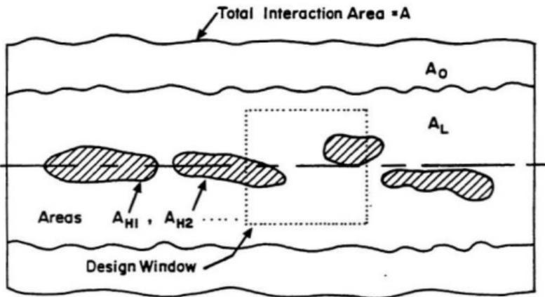
Figure A.3 Critical Zones of High Pressure  $A_{H1}$ ,  $A_{H2}$ , ... and Design Window (Jordaan et al., 1993).
