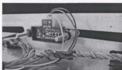
Figure 5.33: Infrared Proximity Sensor Mounted onto Plate
