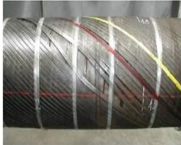
Figure 6-1. Cross section of unbounded flexible pipe [2].
