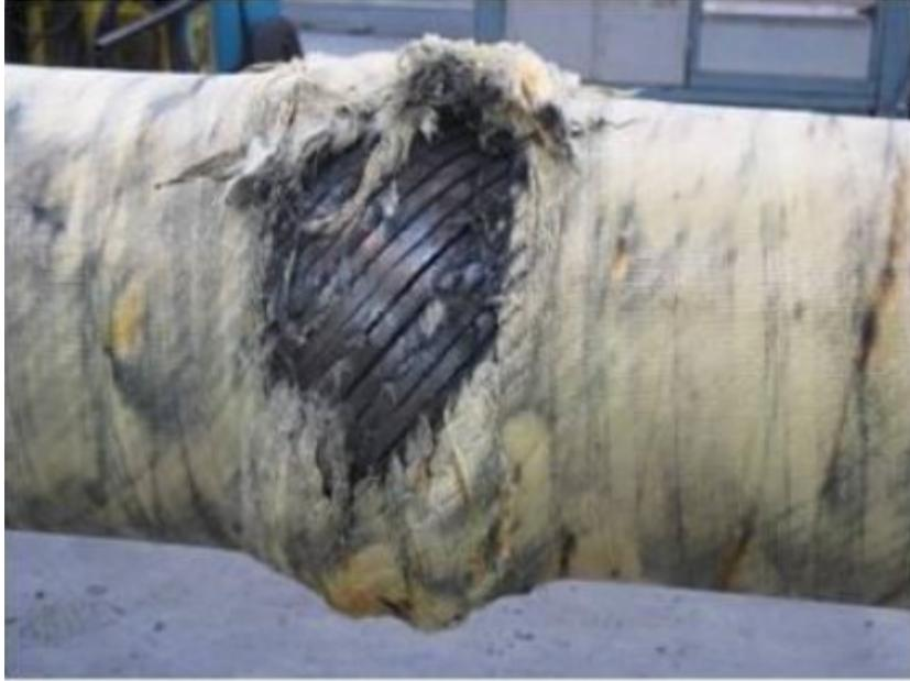
Figure 1-2. Radial buckling (Birdcaging) in flexible flowline. Secher *et al.* [14].
