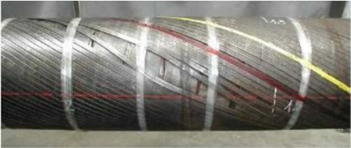
Figure 1-3. Lateral buckling in flexible flowline, Secher *et al.* [14].
