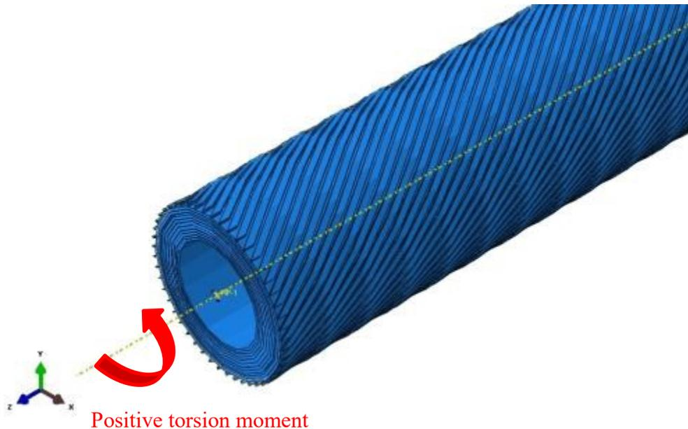
Figure 4-3. Direction of positive twist moment which tend to untwist the external tensile armours.
