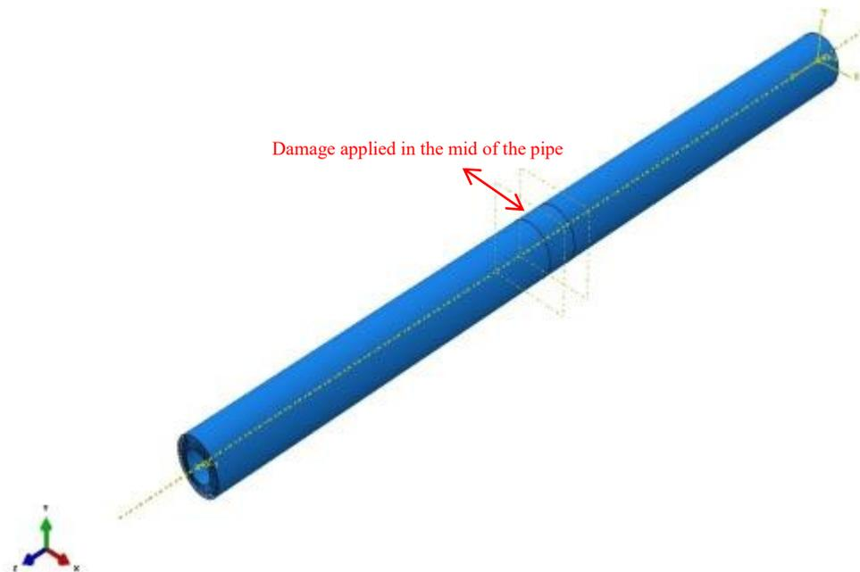
Figure 3-18. Damaged area applied in the middle of pipe length.
