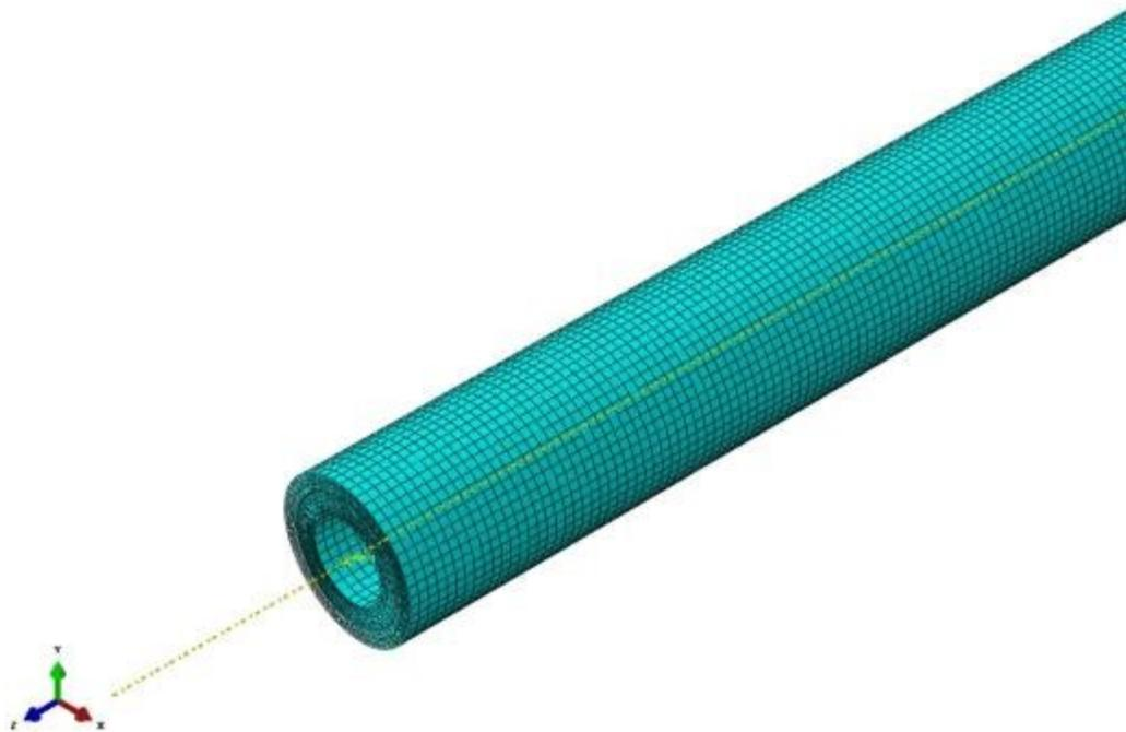
Figure 3-1. Layers and element distribution in the cross section
