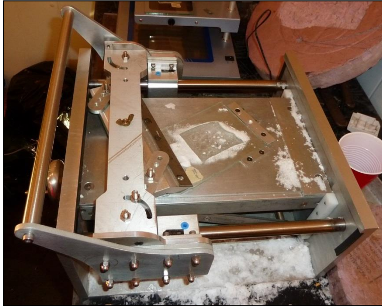
Figure 3.11: Image of manually operated microtome to machine thin ice sections.
