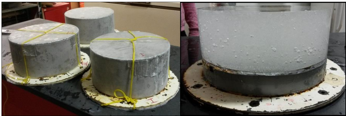
Figure 3.2: (Left) Ice holder - aluminum bucket setup to grow ice specimen. (Right) Ice holder with unprocessed cylindrical specimen.
