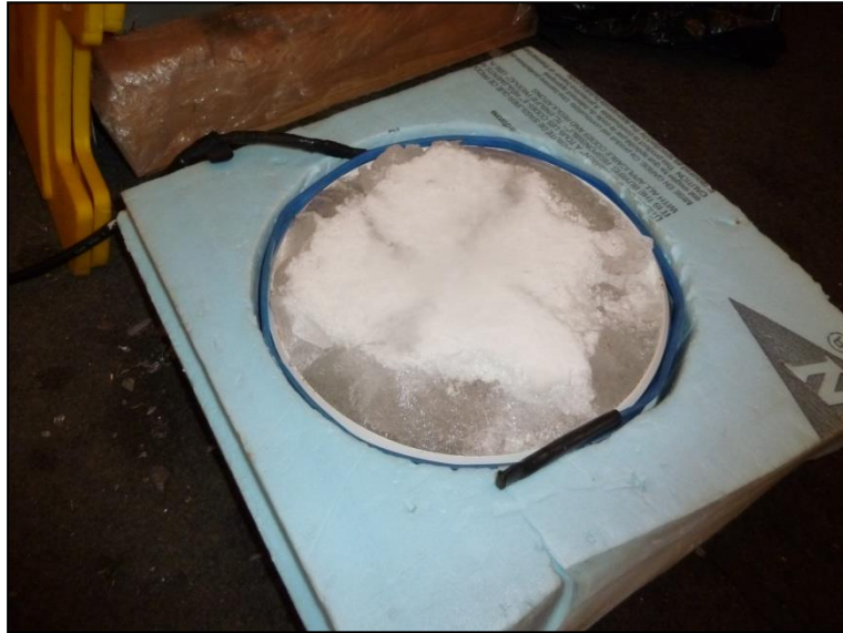
Figure 3.10: Picture showing an ice specimen with a warm wire winded around for detaching it from the mold.
