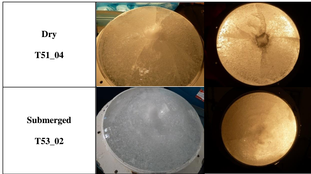
Figure 5.74: Sphere, 100 mm/s, 20° ice specimens: images of ice samples after testing in dry (top) and submerged (bottom) contact conditions; on the left of indented surfaces, on the right with lighting applied from the back.
