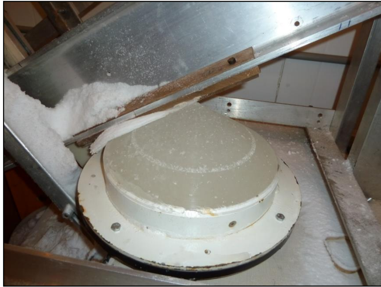
Figure 3.3: Ice shaping apparatus to machine conical ice specimen.
