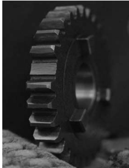
Fig. 4. B4 gear with the broken tooth.
