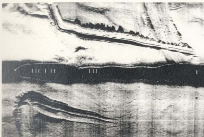
Figure 1.1 500 kHz sidescan sonar image (swath width 75 m) showing ice scour features at 15 to 25 m water depth interval in Resolute Bay (courtesy of the Atlantic Geoscience Centre)
