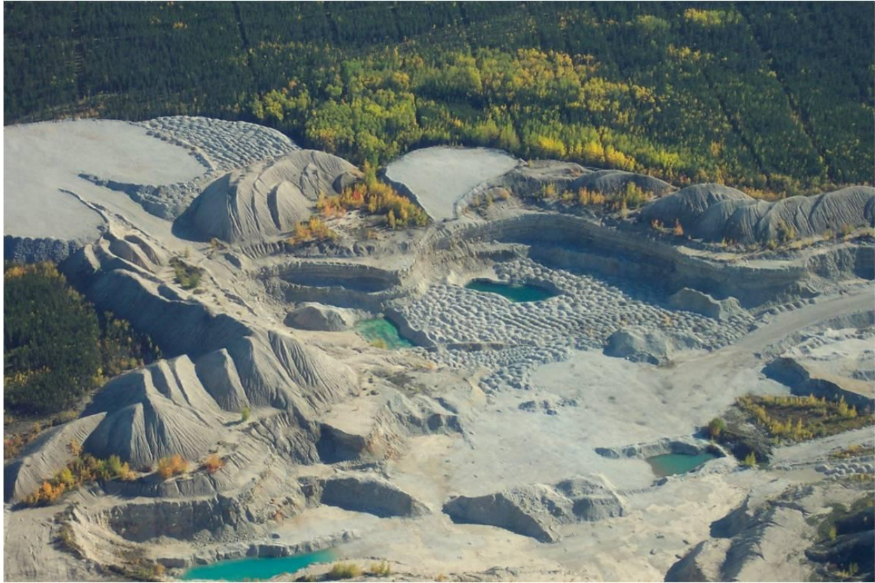
Figure 1. 2 Oblique aerial photo of a small part of the mine site showing piled waste rock, little vegetation growth, and vertical cutlines through the surrounding forest, ca. 2003. Photo credit: Deninu Kue First Nation
