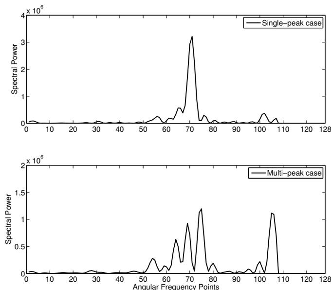
**Figure 2.** The power distribution at different frequency points for two adjacent wavenumber vectors. The upper sub-plot has only one prominent peak, and the corresponding frequency is retained as an element in the dispersion shell. The lower sub-plot shows multiple peaks that are noise contaminated and is thus discarded.
