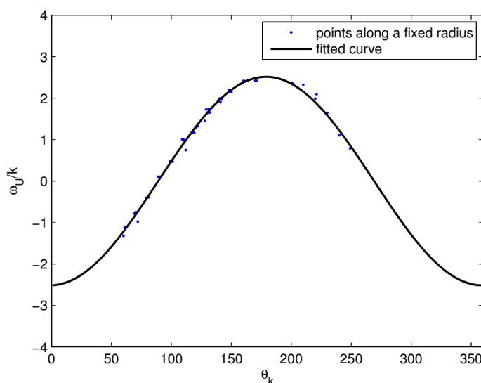
**Figure 3.** The curve fitting process along a particular radius. A clear sinusoidal function is estimated from the input data points, and the peak is seen to have a value close to the input current speed (2.5 m/s) and is located at 180 degrees (measured clockwise from true north), which is exactly the input current direction.
