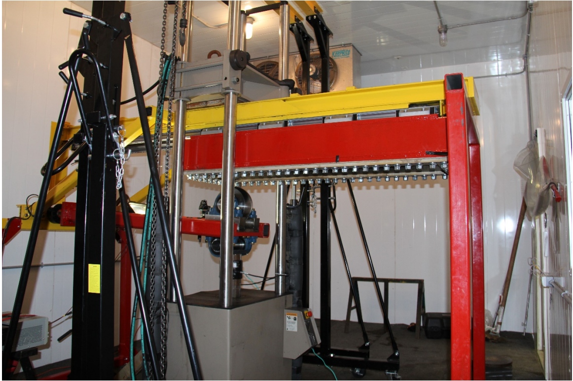
Figure 3.4: Moving load apparatus housed in a cold room.
