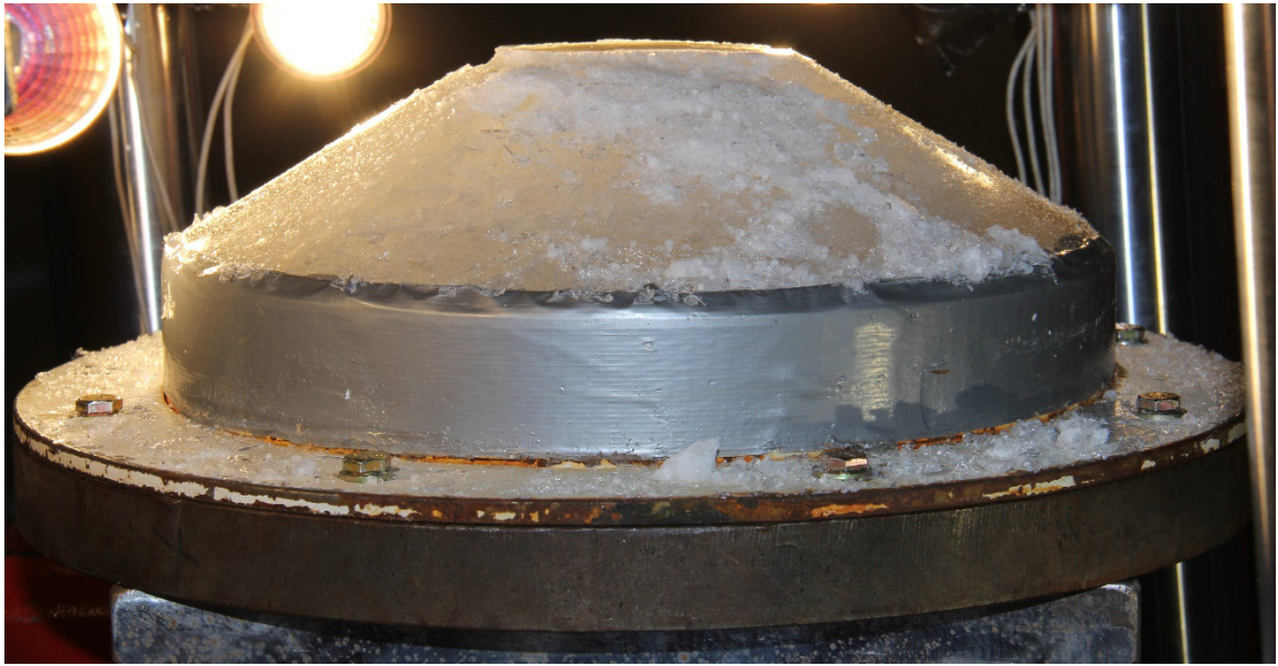
Figure 3.12: Example ice cone indenter after test – crushed surface (truncating surface of the ice cone) and extruded ice (snow like substance on the surface of the ice cone and indenter) are apparent.
