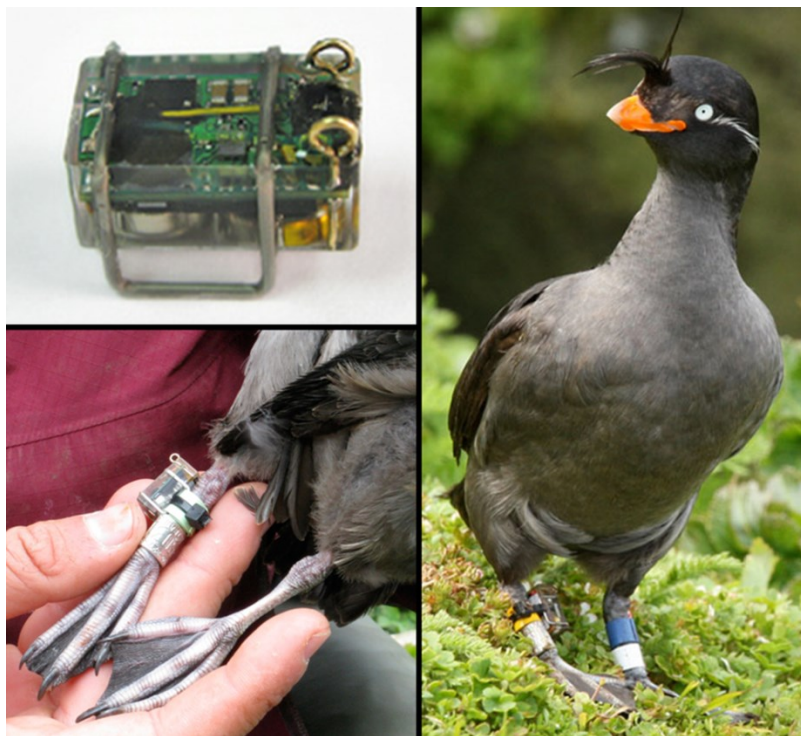
Figure 2.1: Photograph of Lotek Wireless, Lat-2900 Series Avian Geolocator and placement of device attached to an adult Crested Auklet at Buldir Island Alaska.
