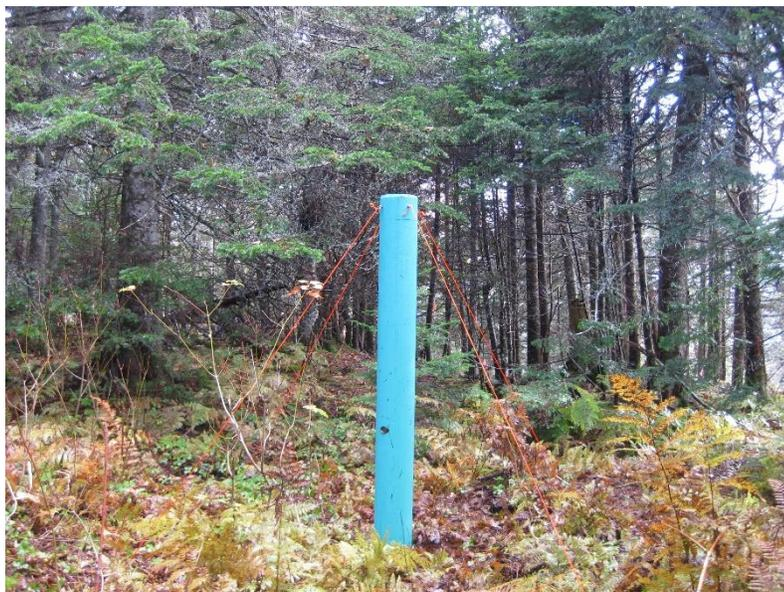
**Figure 3.** Static precipitation sampler field setup.
