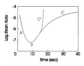
Figure 3.8 Illustration of strain rate history of ice. A: Decelerating creep; B: Minimum creep rate; C: Accelerating creep; C': Run-away behaviour.
