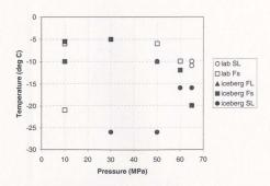
Figure 3.11 P-T relationship for specimens showing different types of failure: SL, Fs and FL represent strain localization, shear fracture and axial splitting, respectively.
