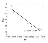
Figure 4.4a ln(\$\phi\$) against 1/T at pressure = 70 MPa after the first correction
