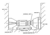
Figure 3.2 Schematic of the actuator indentor system (Frederking et al. 1990a)
