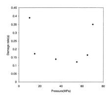
Figure 4.5 Damage rate( $\phi$ ) plotted against hydrostatic pressure at -10°C after temperature correction for the first calibration
