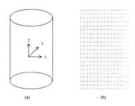
Figure 5.3 (a) Ice cylindrical specimen; (b) Mesh for a specimen
