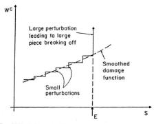
Figure 2.9 Growth of damage S and change in complementary strain energy W (Jordan and Xiao, 1992).
