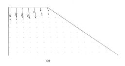
Figure 6.7 Energy flux evolution history: (a) time =  $0.02 \, s$ ; (b) time =  $0.048 \, s$ ; (c) time =  $0.05 \, s$ .
