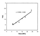
Figure 4.10 Natural logarithm of damage rate,  $\phi$  versus stress at pressure = 55 MPa
