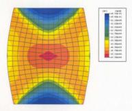
Figure 5.5c Damage contour plot for pressure = 60 MPa
