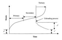
Figure 2.1 Strain history curve of ice under constant stress conditions.
