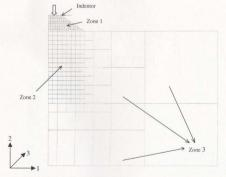
Figure 6.2 Mesh of the indentation model.
