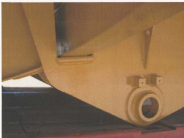
Figure 6-2: DT-HiLoad Body Design - Close-up of Floor Stiffener Intersection
