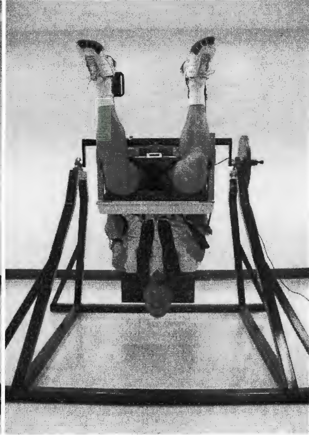
Fig 3.1b Inversion Chair Apparatus demonstrating inverted seated posture.
