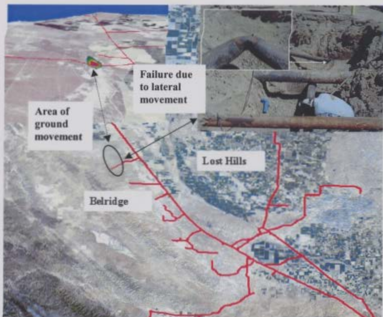
Figure 4-1: Pipeline failure due to lateral ground movement. (Courtesy of Southern California Gas Company and C-CORE)
