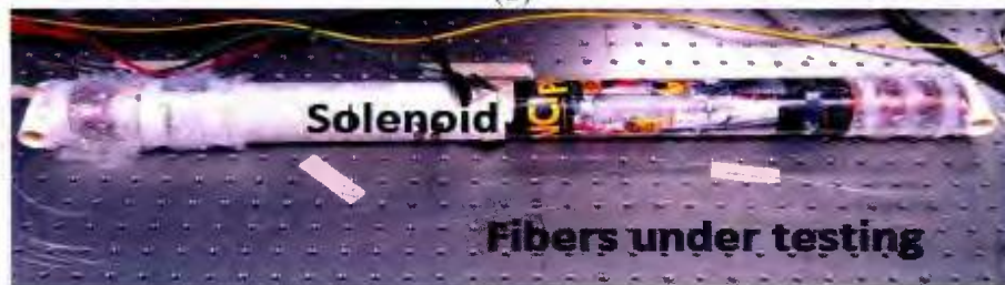
Figure 1-4 Principle of FOCS: (a) principle of Faraday magneto-optic effect; (b) principle of Ampere circuital theorem; (c) an actual FOCS
