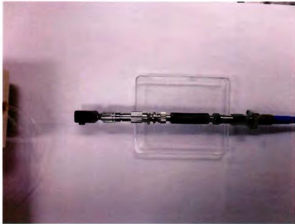
Figure 3-23 A pre-polarizer is deployed to obtain an ideal initial linear input SOP
