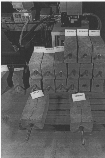
Fig. 6.25 Specimens with rebar diameter of 35 mm after cyclic test
