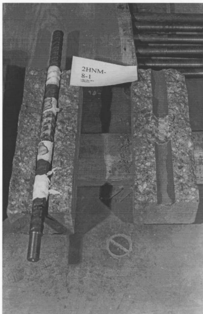
Fig. 5.28 High strength concrete specimen without confinement after pull out test
