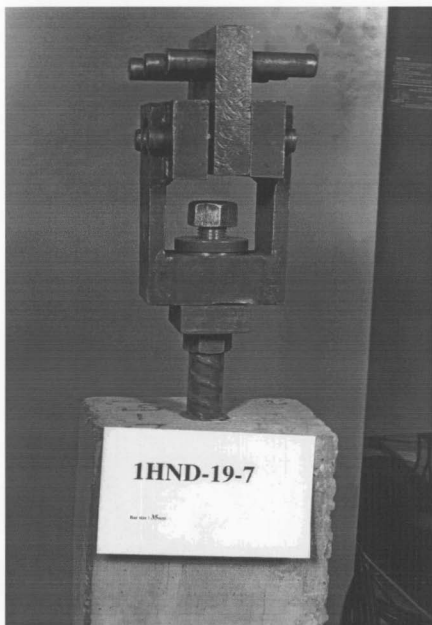
Fig. 4.7 Cyclic specimen after testing
