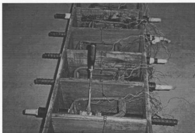
Fig. 4.4 Concrete strain gauges glued around rebar prior to casting
