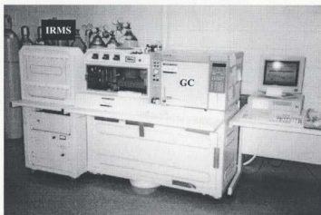
Fig. 2.2. Gas chromatography continuous flow isotope ratio mass spectrometer (GC-IRMS) of the Isotope Biogeochemistry Laboratory, Department of Earth Sciences, Memorial University.
