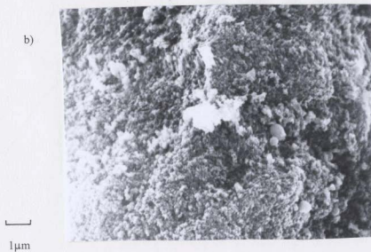
Figure 4.14 SEM Micrographs of Char Carbonized (a) at 600 °C and (b) at 900 °C
