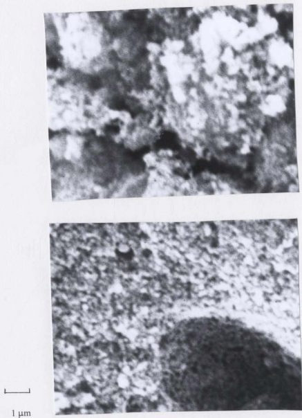
Figure 4.16 SEM Micrographs of Char Blended with 20 % Molasses Followed by Activation Using Steam
