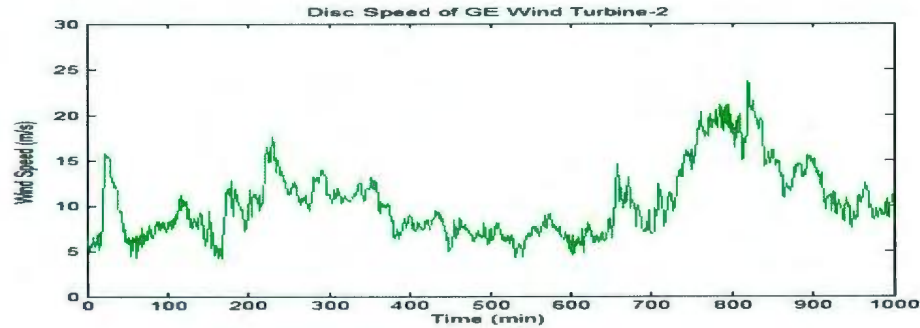
Figure 4.17: Estimated disc Speed (adjusted for turbulence and shear) for GE 1.5 MW wind turbine-2 at hub height. (Note: Time Scale: X axis: 1 unit=10 minute; 1000 unit = 10000 minutes).
