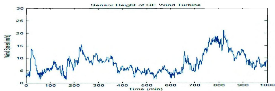
Figure 4.11: Sensor height wind speed data for the GE 1.5 MW wind turbine-2 recorded from MET tower1. (Note: Time Scale: X axis: 1 unit =10 minute; 1000 unit = 10000 minutes).
