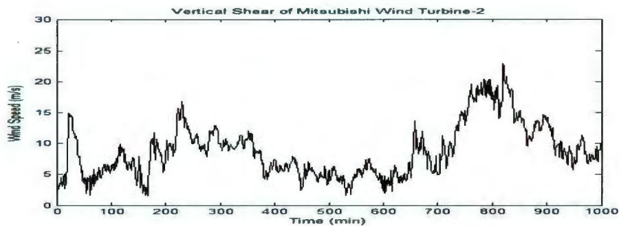
Figure 4.14: Hub height wind speed estimated for the Mitsubishi 1MW wind turbine- 2. (Note: Time Scale: X axis: 1 unit=10 minute; 1000 unit = 10000 minutes).
