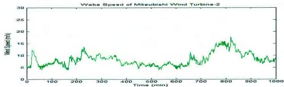
Figure 4.20: Wake speed estimated for Mitsubishi 1.0 MW wind turbine-2 at hub height. (Note: Time Scale: X axis: 1 unit = 10 minute; 1000 unit = 10000 minutes).
