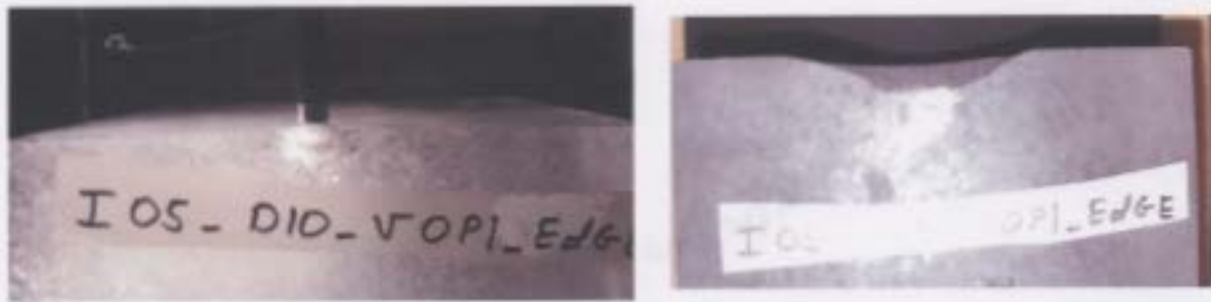
Figure Error! No text of specified style in document.-5: I05_D10_V0p1_E- Post test pictures. This set of pictures illustrates well the zone of damage under the indenter.
