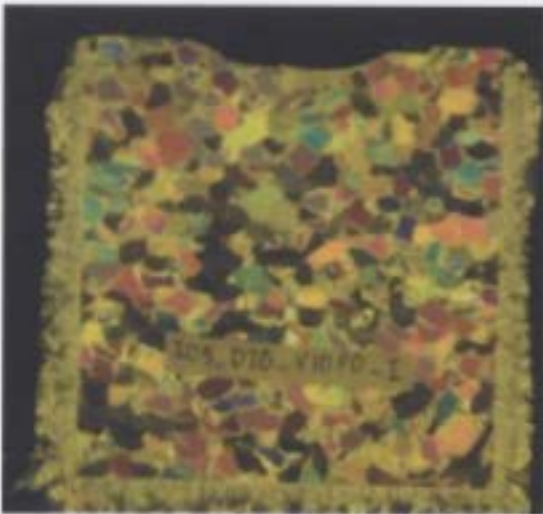
105_D20_V10p0_I- Thin section pictures (indented from top). The left side shows the thin section under cross polarized light. The right side shows the thin section under a side reflected light.
