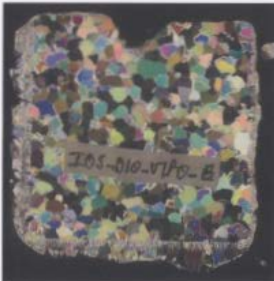
105_D10_V1p0_E- Thin section pictures (indented from top). The left side shows the thin section under cross polarized light. The right side shows the thin section under a side reflected light.
