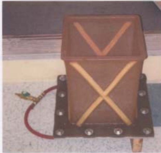
Figure 4-8: Polycrystalline ice block mold. (Note: the hose and valve to the left, used for vacuuming out air, and flooding with de-aerated water.
