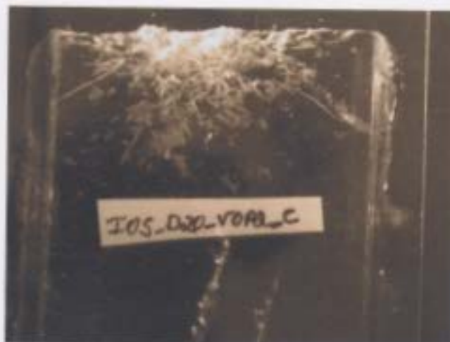
I05_D20_V0p2_C- Thin section pictures (indented from top). The left side is the thin section under cross polarized light and the right side is the thin section under side reflective light. Note the large zone of micro-cracking.
