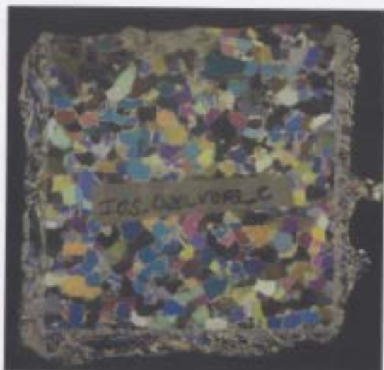
I05_D20_V0p2_C- Thin section pictures (indented from top). The left side is the thin section under cross polarized light and the right side is the thin section under side reflective light. Note the large zone of micro-cracking.
