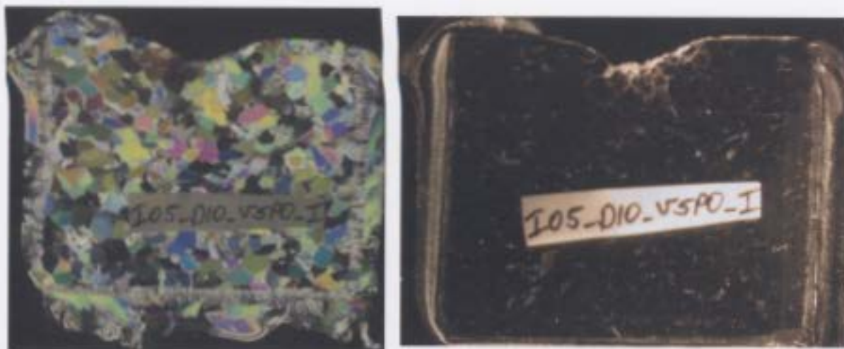
Figure 5-3: I05_D10_V5p0_I -Thin section pictures (indented from top). The left side shows the thin section under cross polarized light. The right side shows the thin section under a side reflected light.
