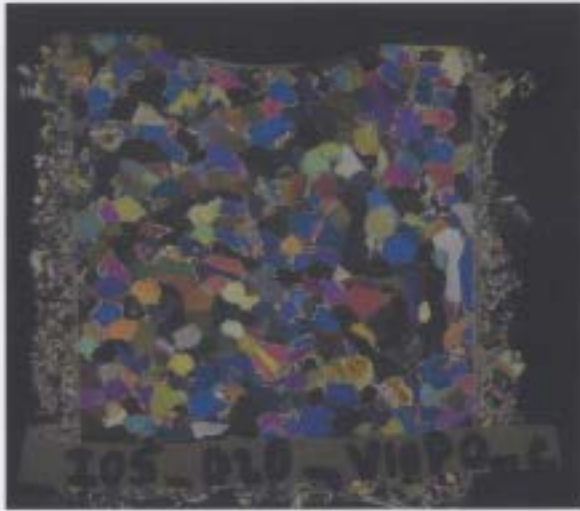
I05_D20_V10p0_C- Thin section pictures (indented from top). The left side shows the thin section under cross polarized light. The right side shows the thin section under a side reflected light (note that the micro-cracks at depth are forming around grain boundaries).
