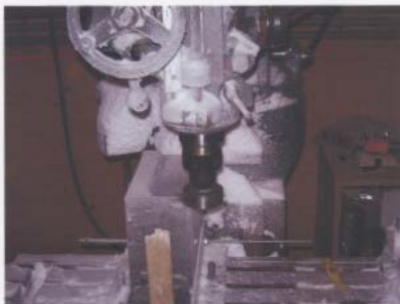
Figure 4-11: Machining test sample using the milling machine in the large cold room at NRC-IOT
