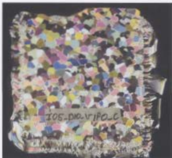
Figure Error! No text of specified style in document.-2: I05_D10_V1p0_C-Thin section pictures (indented from top). The left side shows the thin section under cross polarized light. The Right side shows the thin section under a side reflected light.
