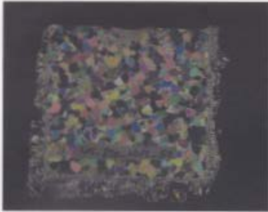
105_D20_V0p2_E2- Thin section pictures (indented from top). The left side is the thin section under cross polarized light and the right side is the thin section under side reflective light. This is a particular good example of inter-grain boundary cracking.
