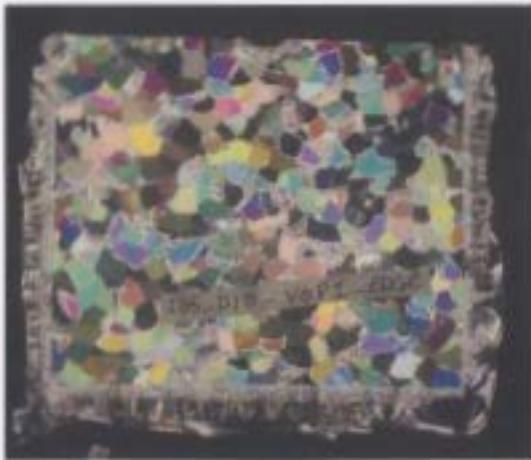
I05_D10_V0p1_E- Thin section pictures (indented from top). The left side shows the thin section under cross polarized light. The right side shows the thin section under a side reflected light.
