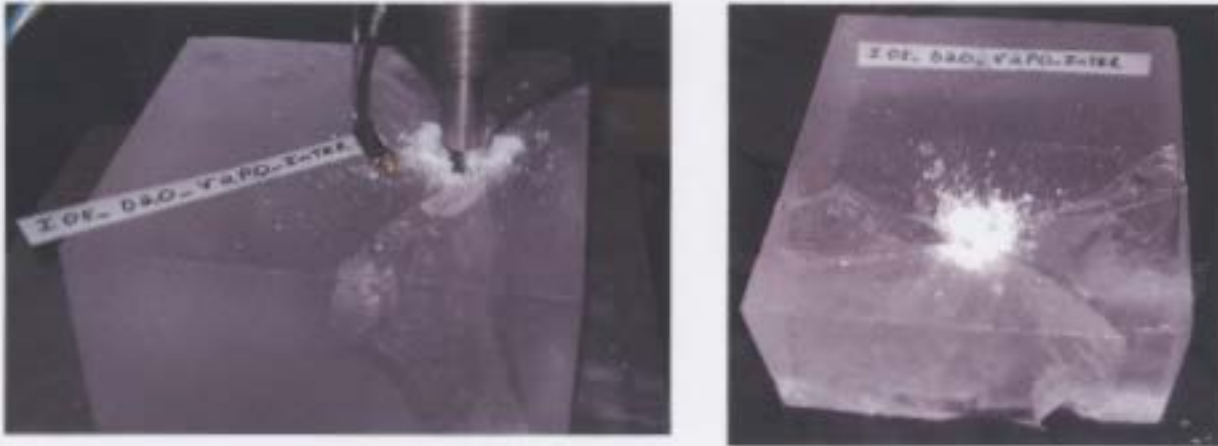
Figure Error! No text of specified style in document.-7: I05_D20_V2p0_I- Post test pictures. This was one of the most violent fractures. Clear and white zones were visible within the indenter footprint even in such a broken test sample.
