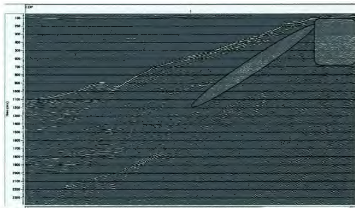
Figure 2.16: The same stack section (a) in Figure 2.15 with pre- and post-stack predictive deconvolution (c). Seabed multiple is traced transparent.
