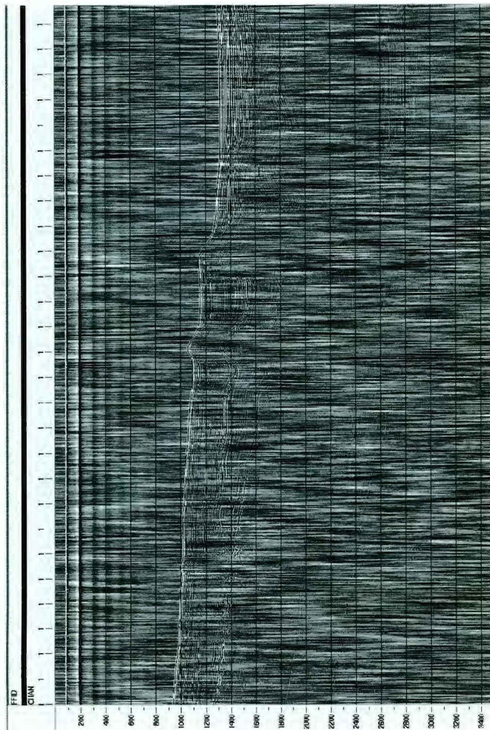
Figure 2.4: Raw data showing a single channel of all shots. The section is noisy and primary energy is not very strong.
