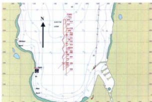
Fig. 4.35 Mission plan for a horizontal and vertical zigzag manoeuvre
