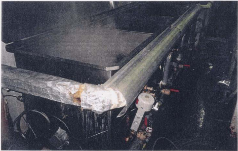
Figure 4: Stainless steel cookers used for cooking rock crab. Heating is accomplished through direct saturated steam injection at the cooker's base through a steam spreader.
