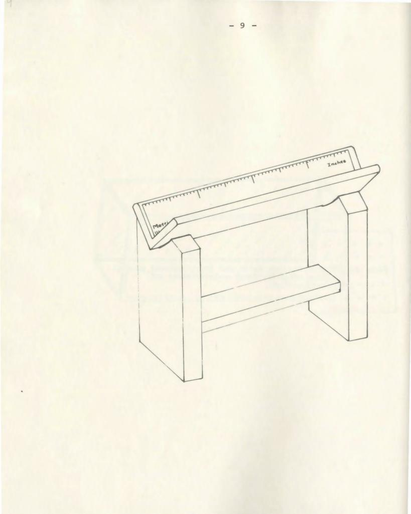
Fig. 2. The V-shaped board for measuring diameter of fish eggs.
