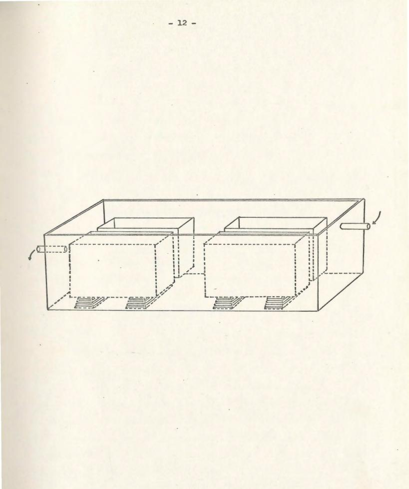
The aquarium tank (Fig. 6) measured 122 cm  $\times$  53 cm  $\times$  35 cm. A six-layer cooling coil containing anti-freeze coolant was placed close to the inner walls of the trough. The coil was connected to a generator with a fan, by means of which the returning, heat-laden anti-freeze was cooled. Water temperature in the tank could be controlled or lowered to a minimum of  $4^{\circ}$ C.
