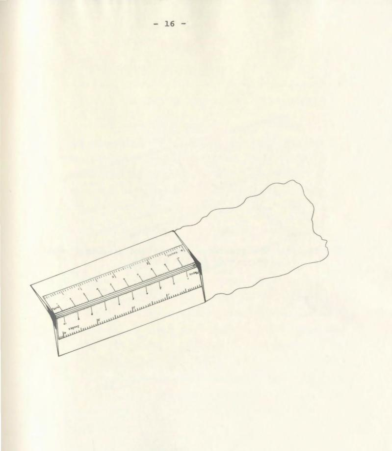
Fig. 8. The aluminium (outer) and plastic (inner) cages used in the stream.
