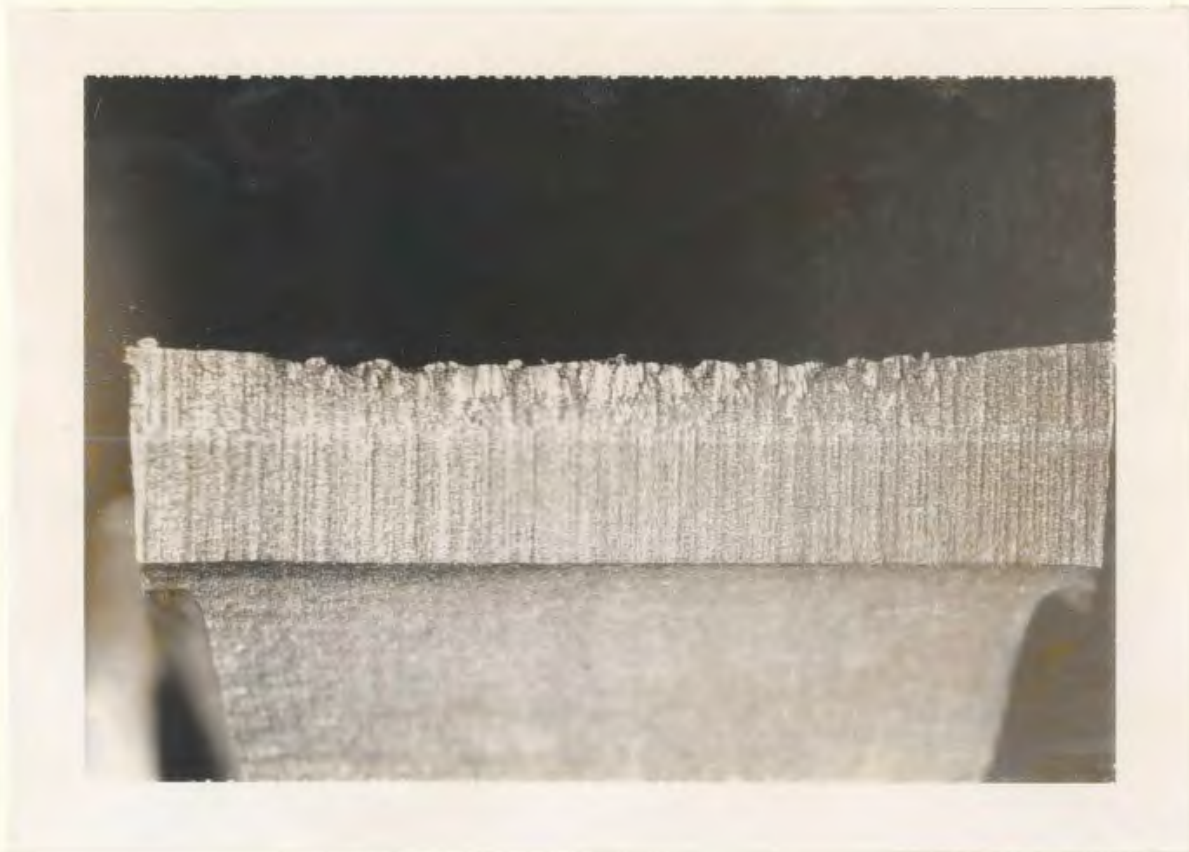
FIG. 6.24 FLANK WEAR ON A CUTTER TOOTH SELECTED AT RANDOM. TWENTY-FIVE CUTS USING COPPER SULPHATE ELECTROLYTE AS A CUTTING FLUID
