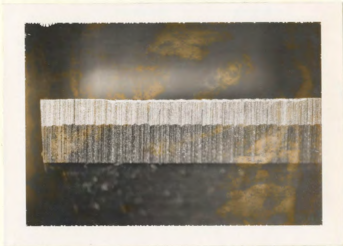
FIG. 6.26 FLANK WEAR ON A CUTTER TOOTH SELECTED AT RANDOM. TWENTY-FIVE CUTS USING SULPHURIZED OIL AS A CUTTING FLUID
