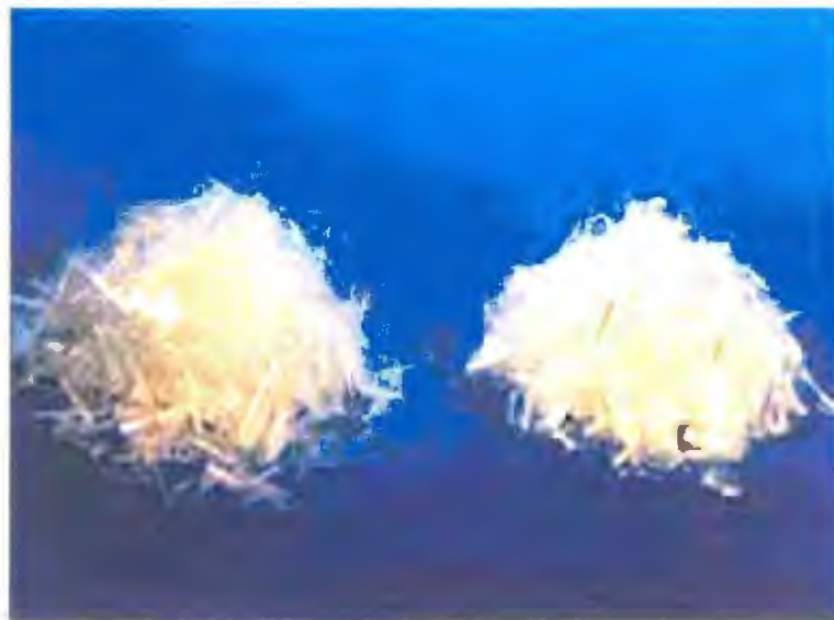
Figure 2.2: Polypropylene fibres are produced either as (left) fine fibrils with rectangular cross section or (right) cylindrical monofilament
