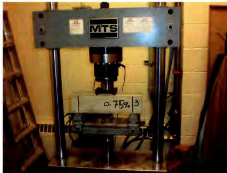
Figure 3.6: Modulus of rupture test setup
