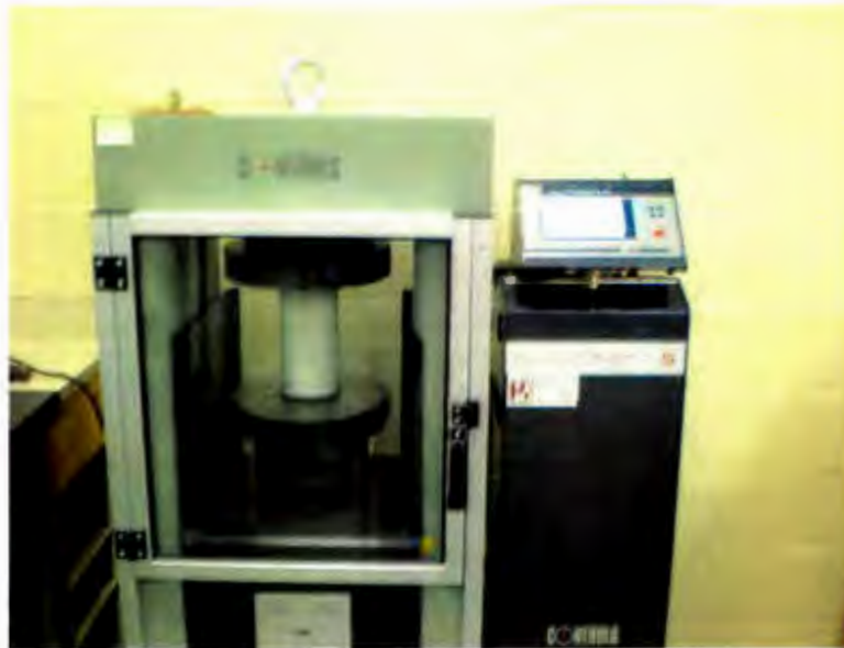
Figure 3.2: Compressive strength test setup
