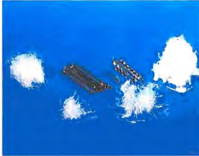
Figure 2.1: Steel, glass, synthetic and natural fibres with different length and shape
