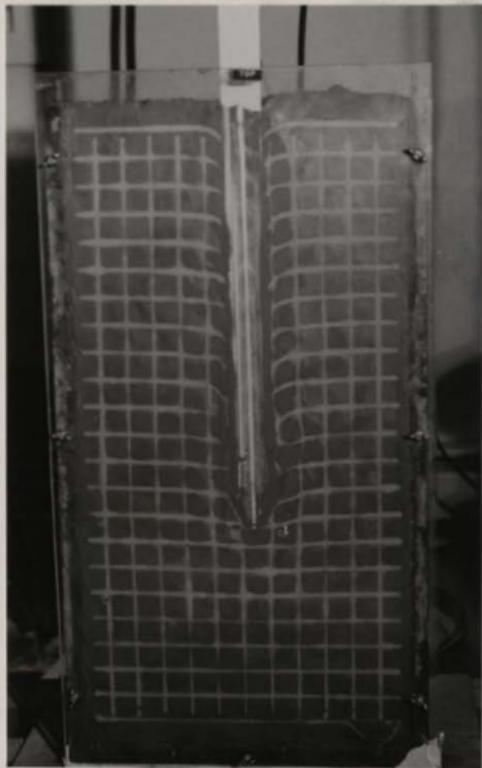
FIG. 15 DISTORTED GRID AFTER HIGH VELOCITY (2.662 FT/SEC)
