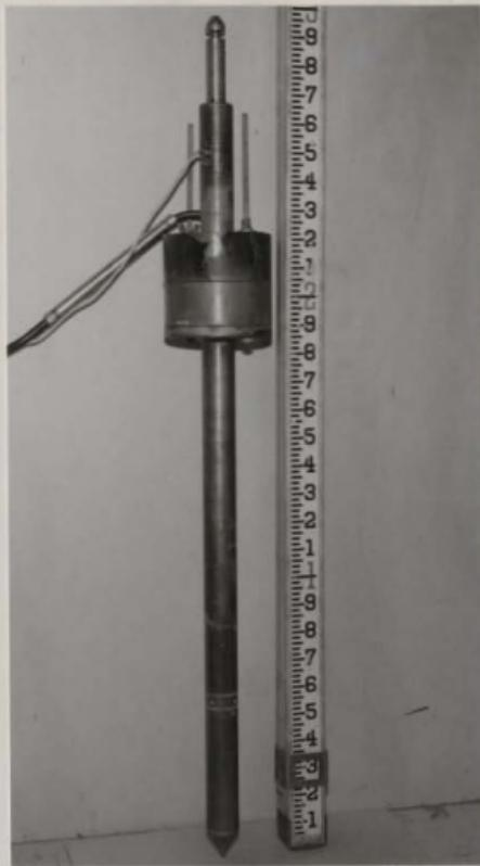
FIG 6 PHOTOGRAPH OF LABORATORY IMPACT PENETROMETER
