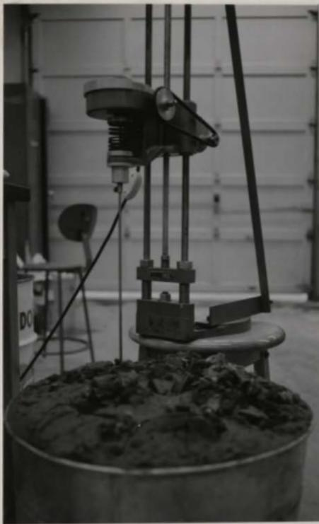
FIG. 10 MODIFIED VANE SHEAR APPARATUS
