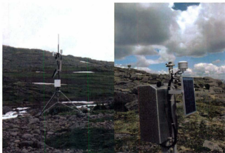
Figure 3.3: Base Station (left photo), elevation 600 m asl; and the Upper Climate Station (right photo) at the summit of Moraine Valley (995 m asl). Note bulk precipitation gauge in the background at the Upper Station.
