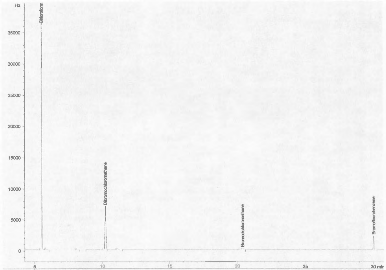
Fig 3.3: Chromatogram of Bonavista tap water sample containing four THM compounds
