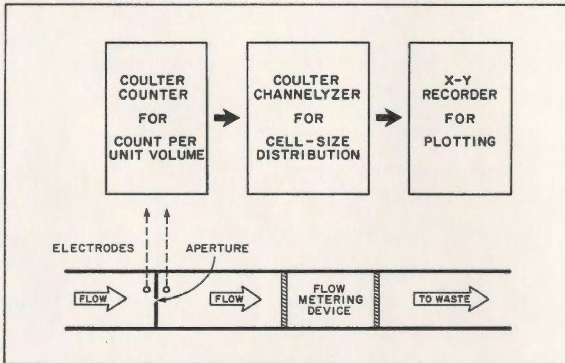
Figure 4: Schematic diagram of the Coulter Counter and Channelyzer (after Wintrobe et al., 1974).
