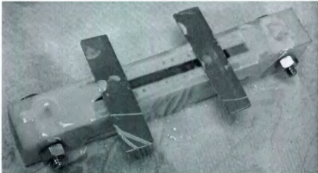
Figure 4-2 Preparation of room temperature vulcanized rubber mould for preparing bending test specimen
