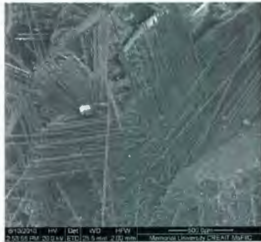
Figure 5-43 Fibre pull out of a bending test specimen after the test.
