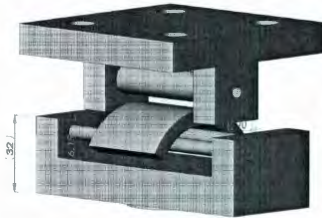
Figure 4-31 Design for three point bending test jig for FRP section
