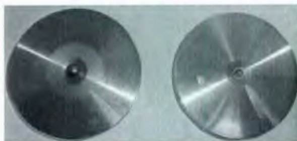
Figure 4-28 Self aligning plate for compression test
