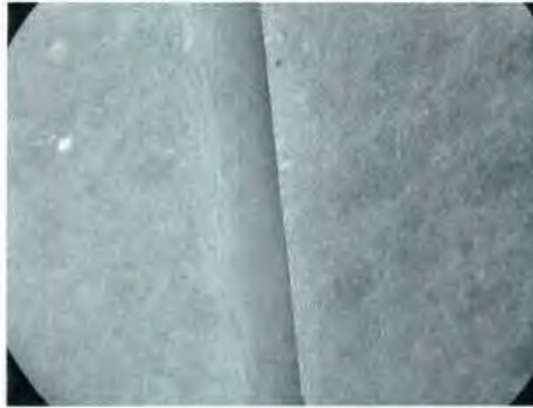
Figure 5-42 Unexposed (left) and exposed (right) surfaces of H150 pipe section.
