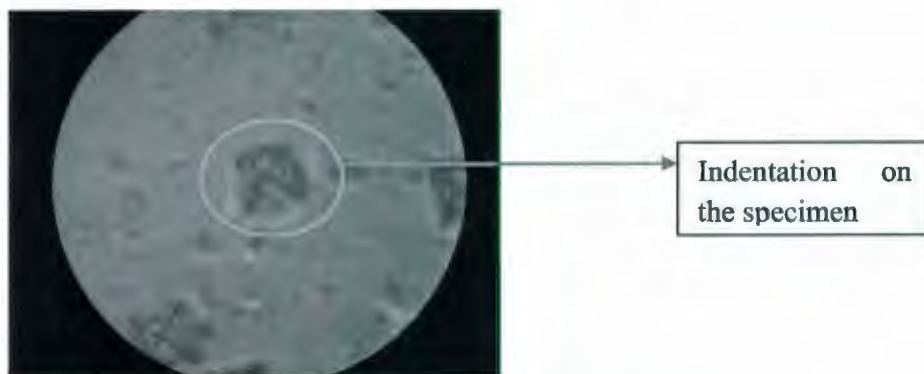
Figure 4-18: 40X magnification of an indentation in the resin
