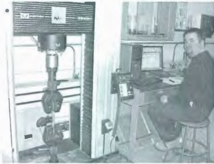
Figure 4-8: Tensile test experiment setup
