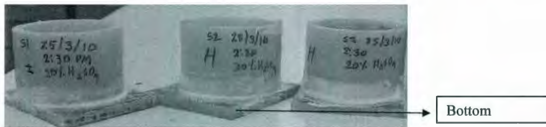
Figure 4-24 H150 specimens prepared for exposing in 1M H 2 SO 4 acid solution
