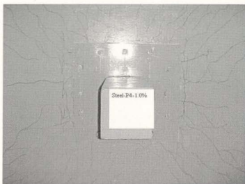
Figure 4.16: Specimen Steel-P4-1.0% after final testing
