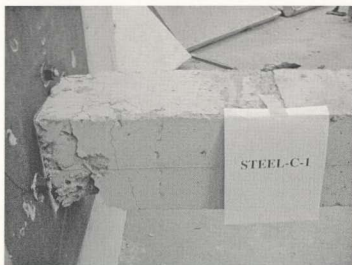
Figure 5.12: Specimen Steel-C-1.0% after final testing.
