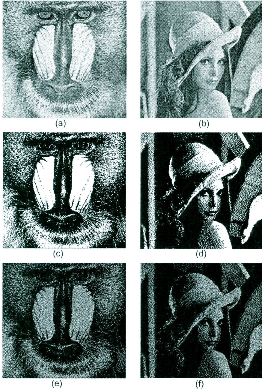
Figure 5.2: Experimental results of multi-image VCS with Chou's method; (a) halftoned baboon; (b) halftoned Lena; (c) processed baboon; (d) processed Lena; (e) reconstructed baboon; (f) reconstructed Lena
