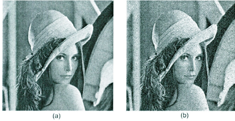
Figure 2.9: Image halftoning with Floyd-Steinberg method: (a) gray scale Lena; (b) halftoned Lena
