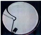
Figure 8: In this image the tank is rotating at the speed \Omega=1.89 rad/s. No flow is induced. Only one colour from the colour slide is being reflected over the entire surface of the rotating fluid. The dark curved line is a barrier placed in the tank.
