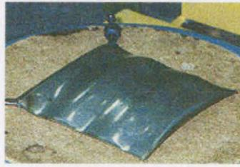
Figure 3.10: Picture of deformed flatjack
