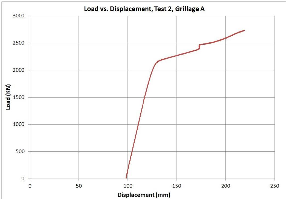
**Figure 2-10: Load vs. displacement, test 2, grillage A**
