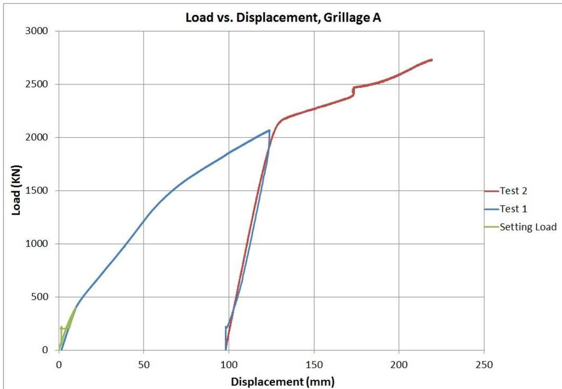
Figure 2-13: Load vs. displacement, grillage A
