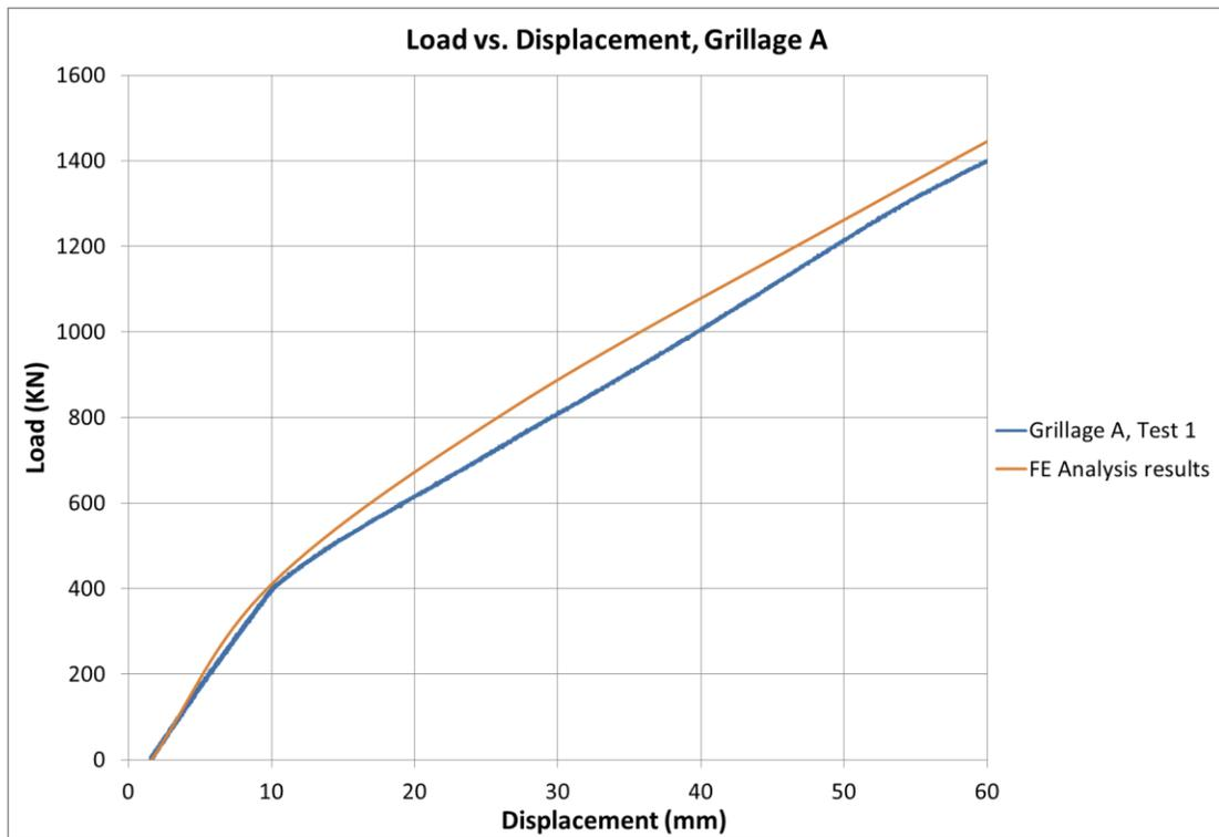
**Figure 3-9: Grillage A, Test 1 laboratory results and FE analysis results up to 1400 kN**
