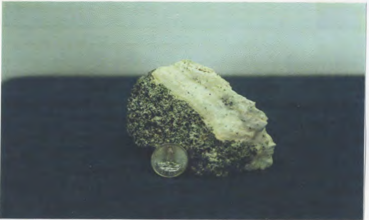
Plate 4.20 Carbonate cave precipitate found within a small cave on the shore section near Loutra tis Aphroditis. Small specks in carbonate are sedimentary clasts. Coin diameter 2cm.
