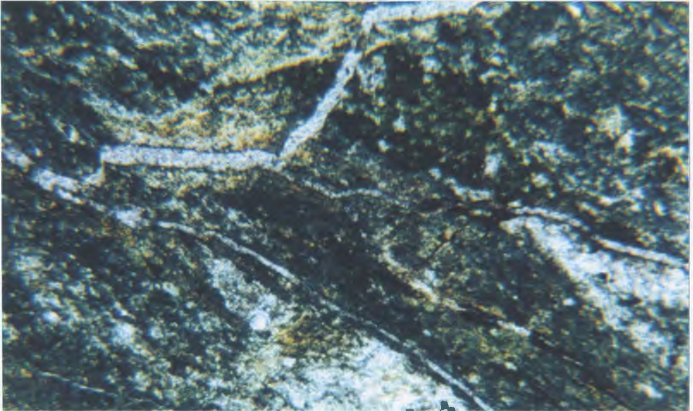
Plate 4.8 Magnesite vein within serpentinitised harzburgite showing brittle deformation. Note specifically cataclastic shear of vein in left bottom quarter of picture. Cross-polarised light. Field of view 3mm.
