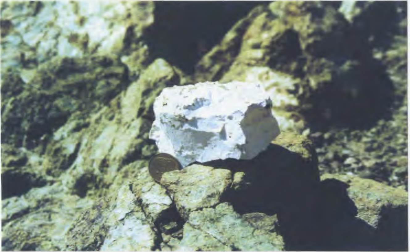
Plate 3.2 Sample of vein magnesite taken from the base of the Magnisia locality. Coin for scale (diameter 10mm).
