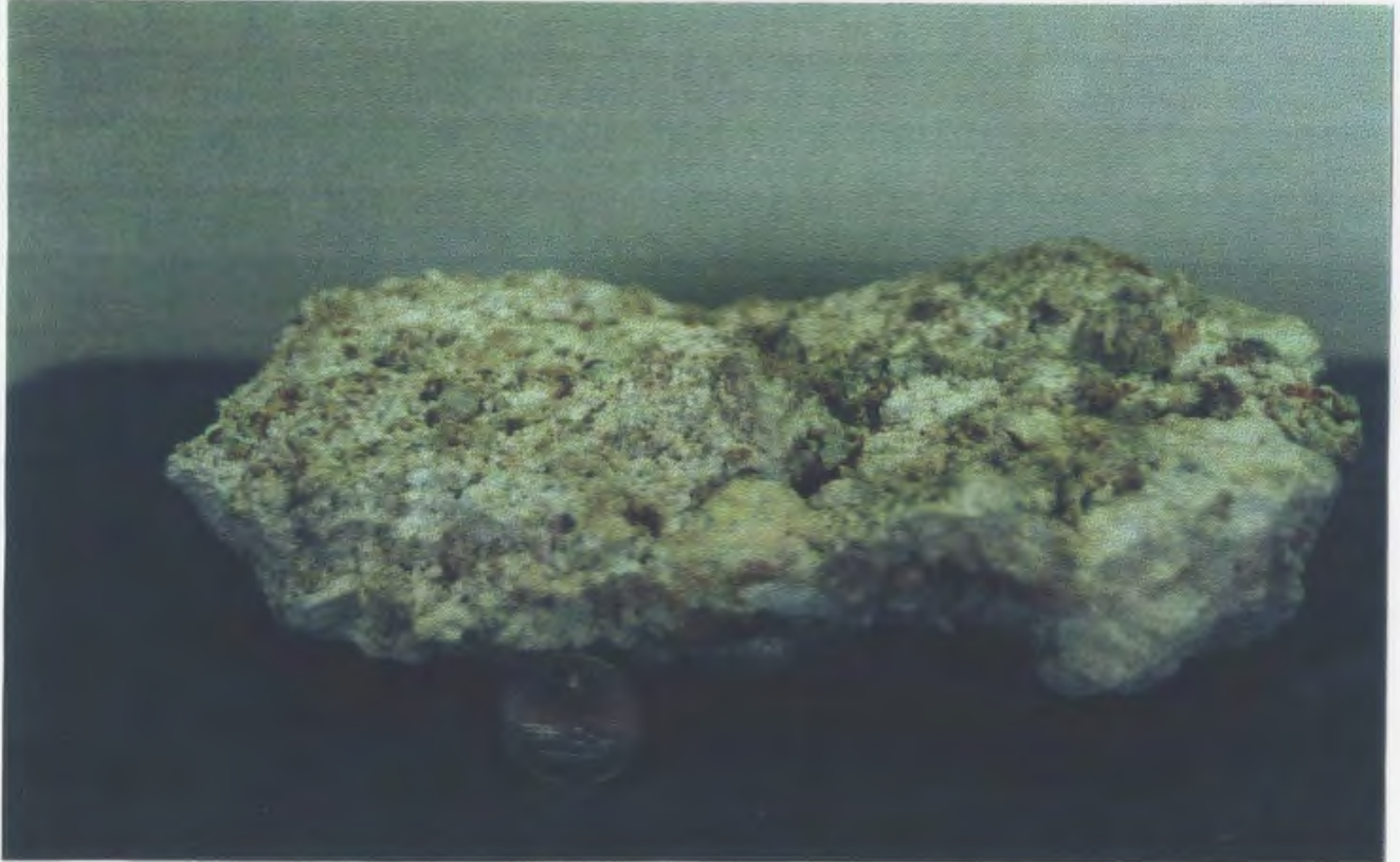
Plate 3.9 A sample of the high-magnesium calcite/magnesite precipitate found on the walls of mining adits in the Magnisia area. Coin for scale.
