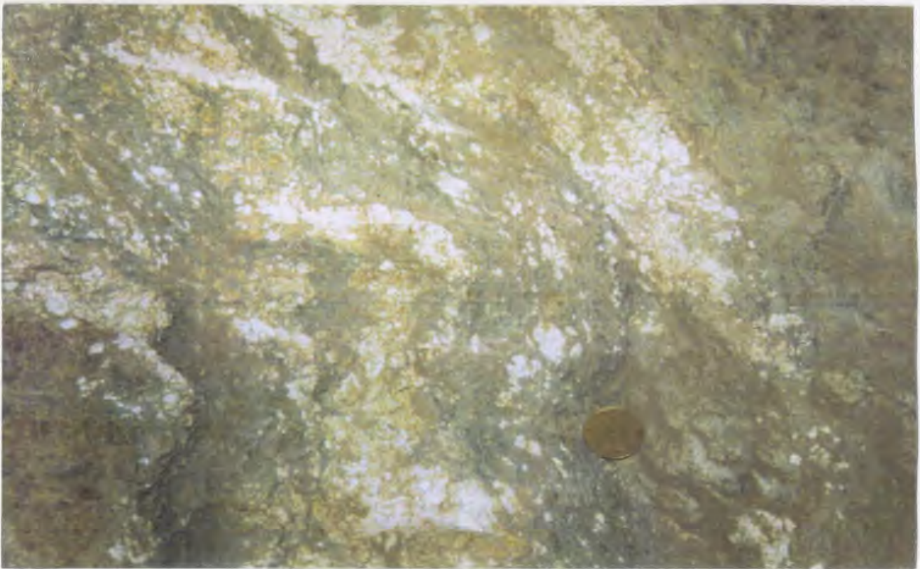
Plate 1.2 Nodular magnesite found throughout the upper portions of the serpentinite.
