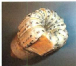
Figure 13. The 1.25-in diamond drag bit
