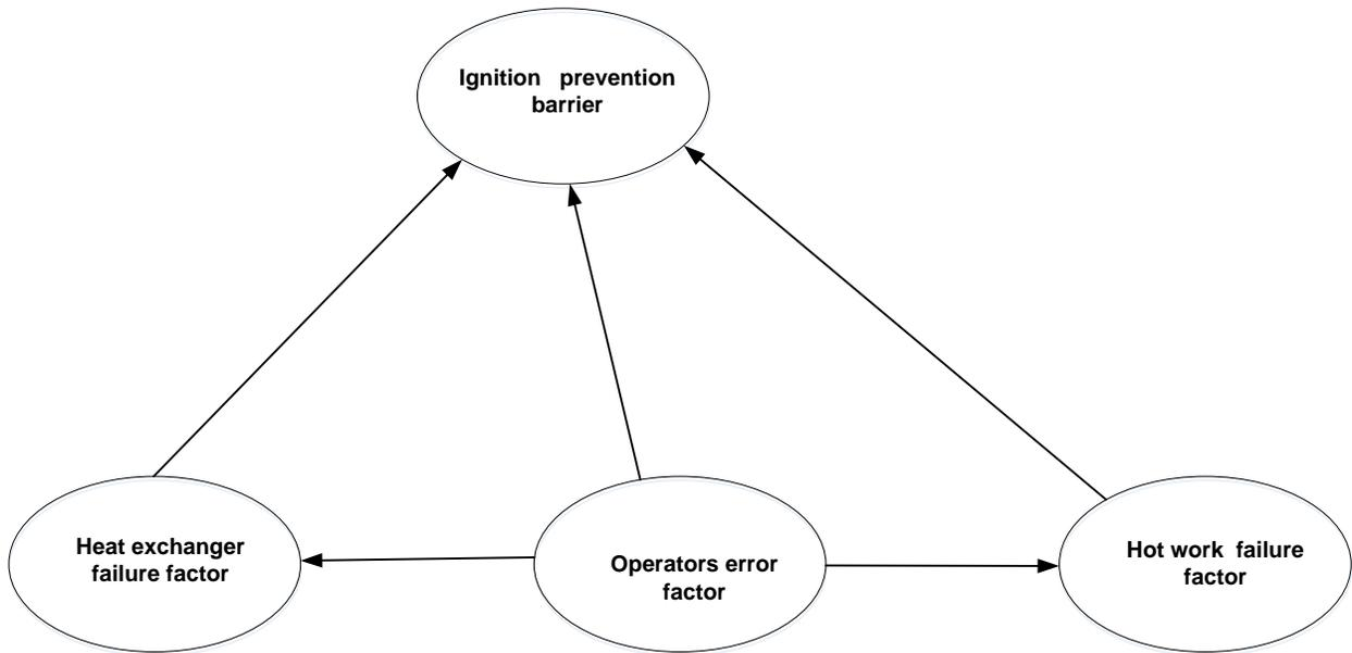
**Figure 5.6 . Interdependency of accident contributory factors in Ignition prevention barrier.**
