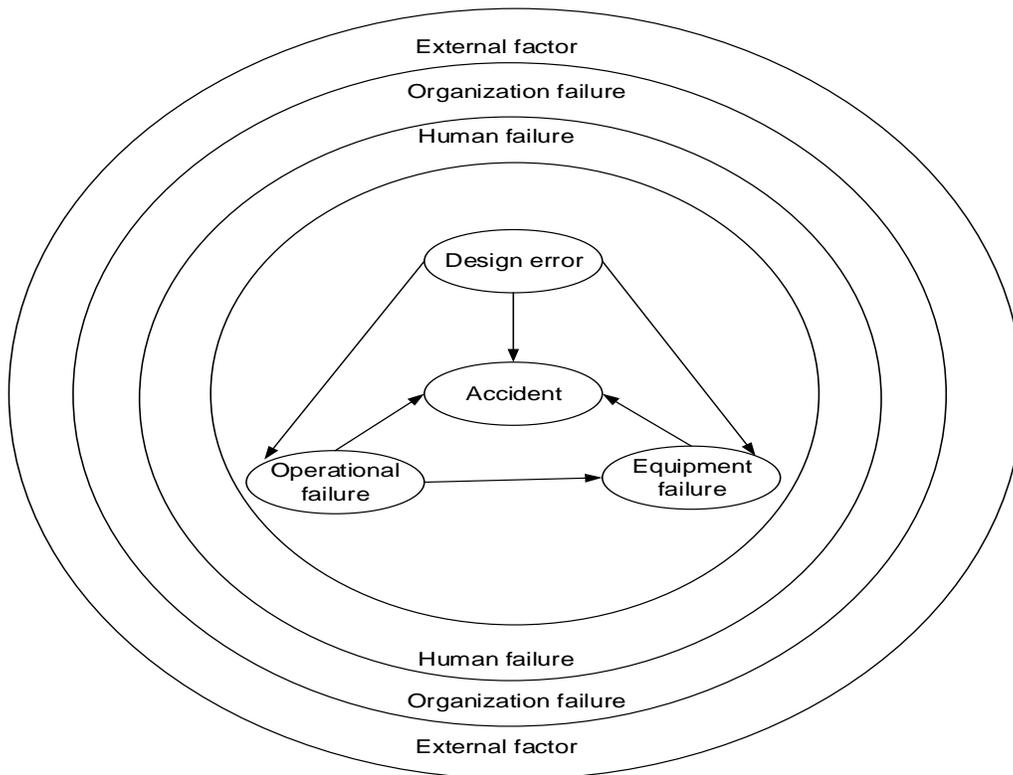
**Figure 4. 2. Interdependency of accident contributory factors in the main model.**
