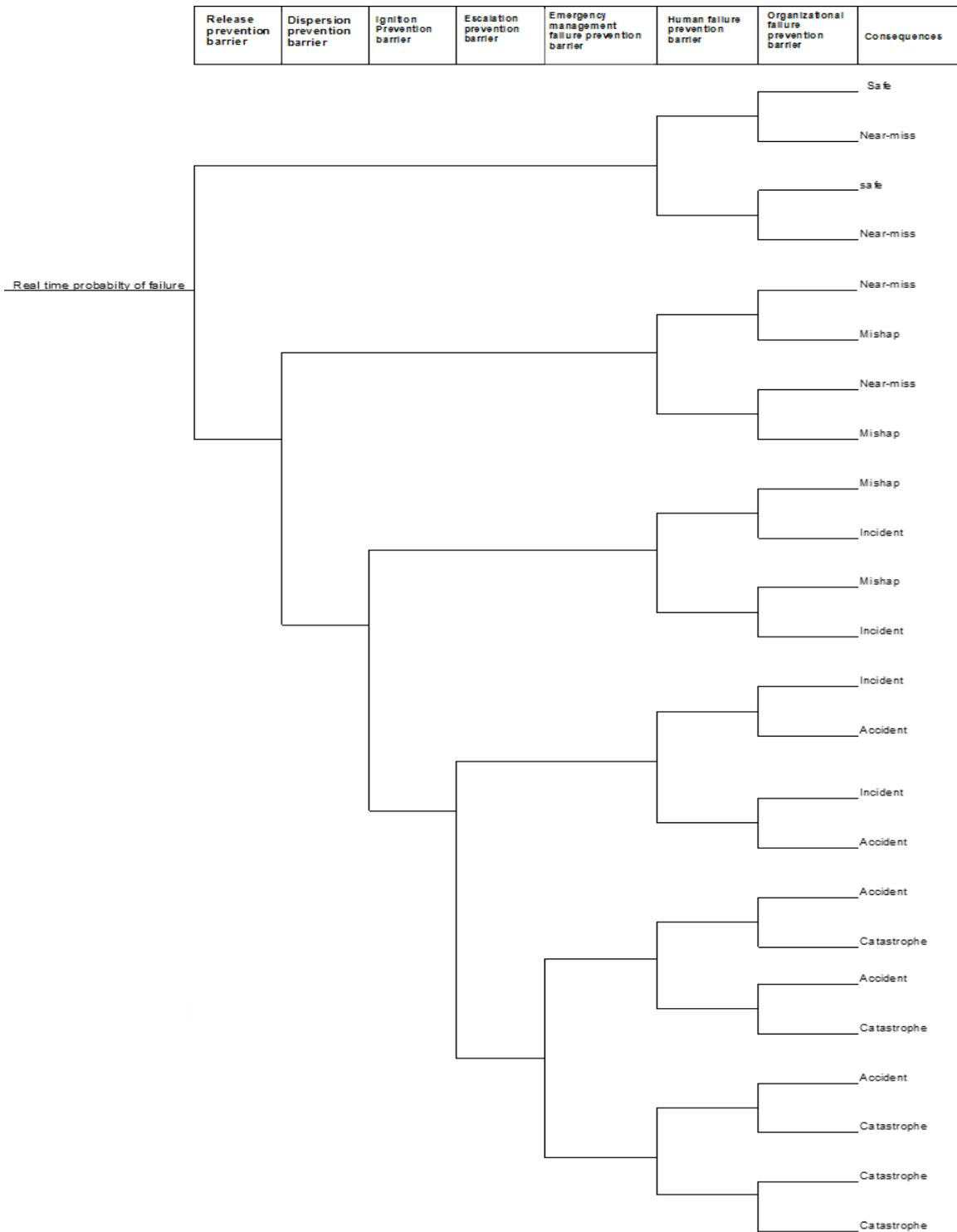
**Figure 6. 4. Revised Event tree for the accident modelling methodology (Adedigba et al. 2016).**
