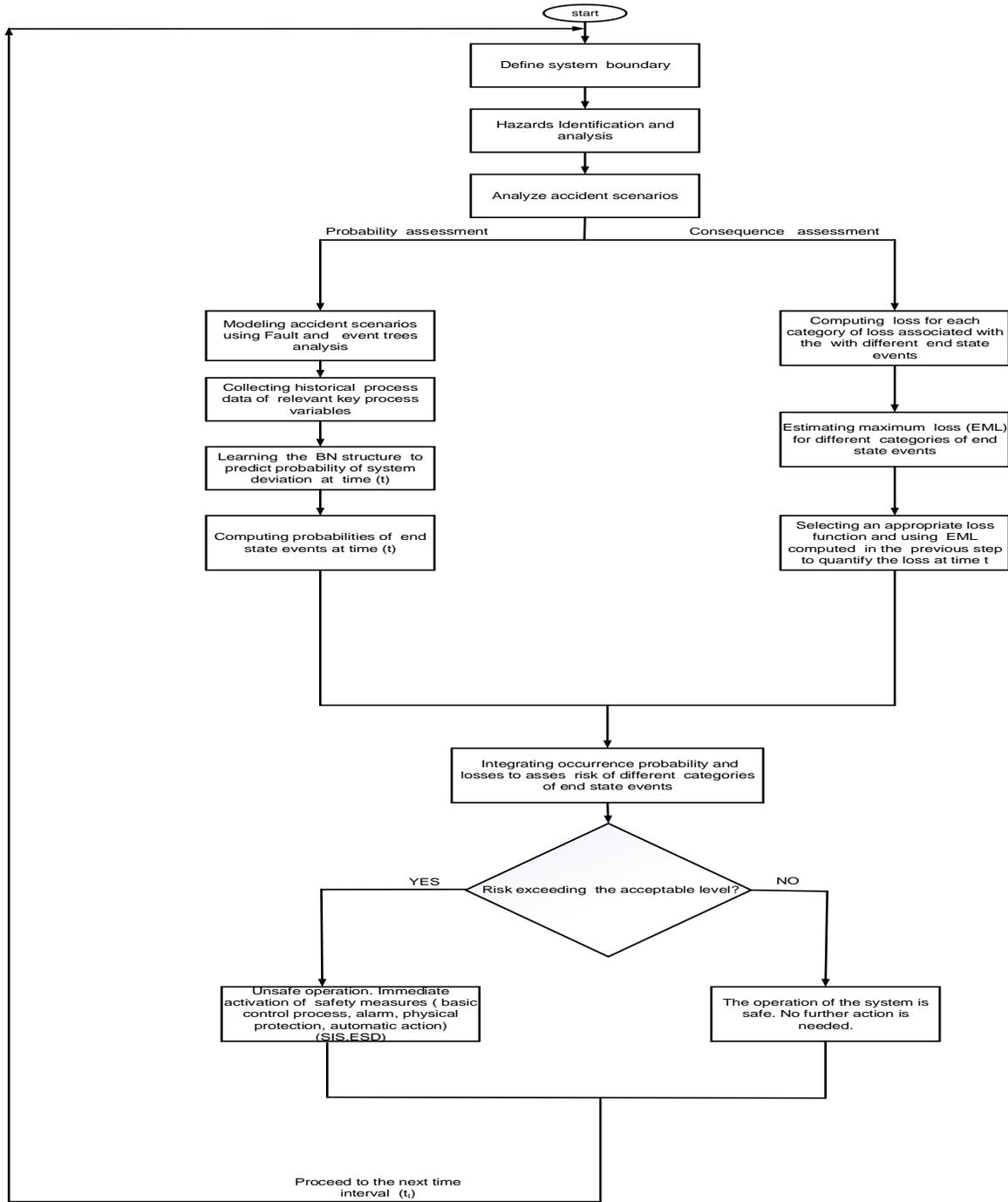
**Figure 8 .1.The flowchart for the proposed methodology.**
