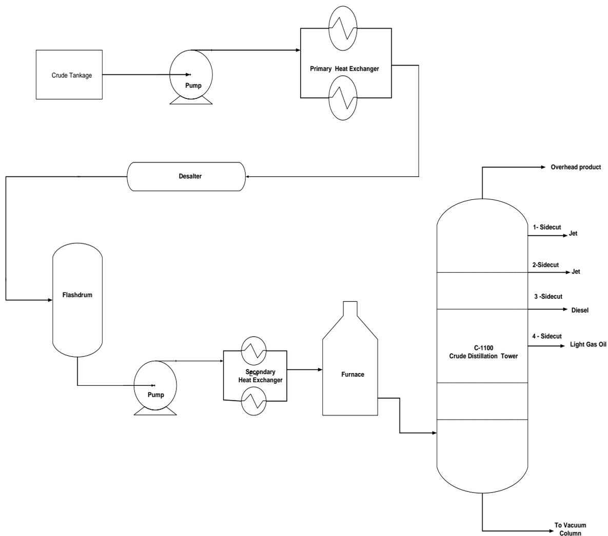
**Figure 8.2. The process flow diagram of Richmond refinery crude unit and its associated up stream equipment( Adedigba et al. 2016; CSB 2015).**
