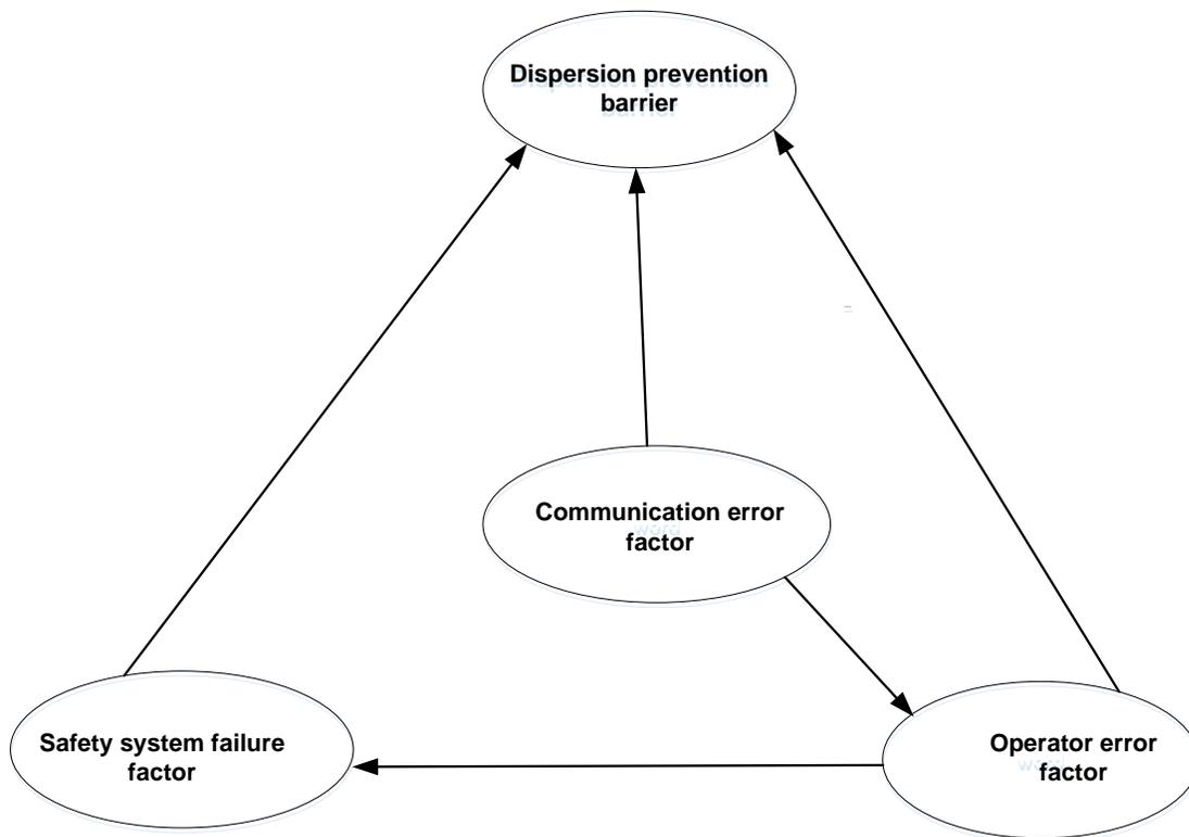
**Figure 5.5. Interdependency of accident contributory factors in Dispersion prevention barrier.**
