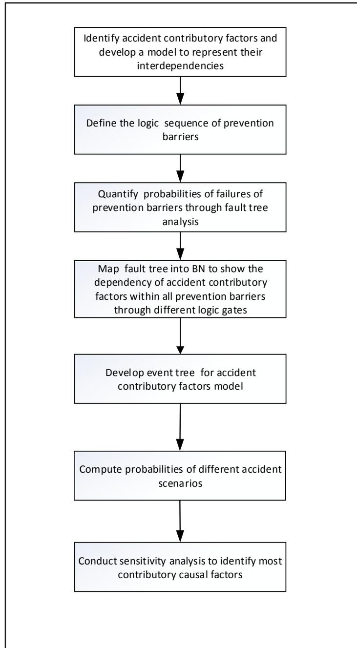
**Figure 4. 1. Flow chart for the proposed accident modeling steps.**
