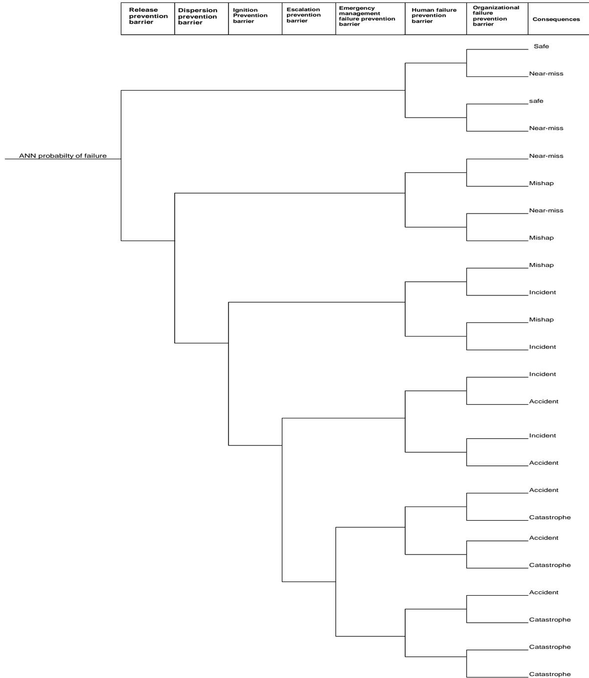
**Figure 7. 4. Event tree for the proposed accident modelling methodology.**
