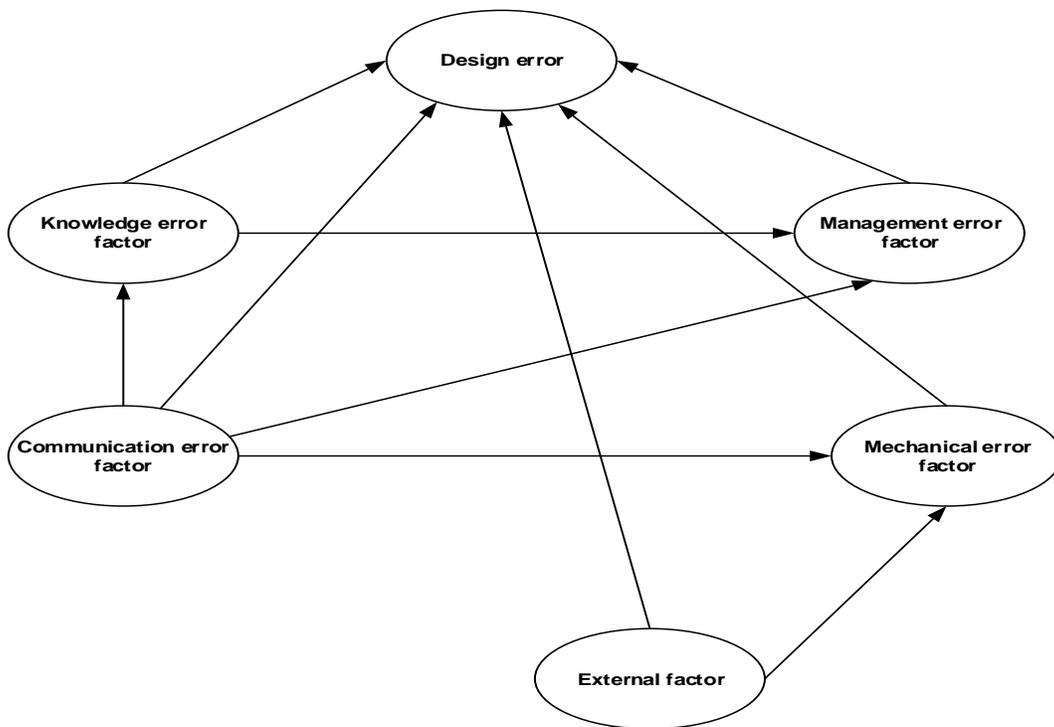
**Figure 4 .4. Interdependency of accident contributory factors in design preventive barrier.**
