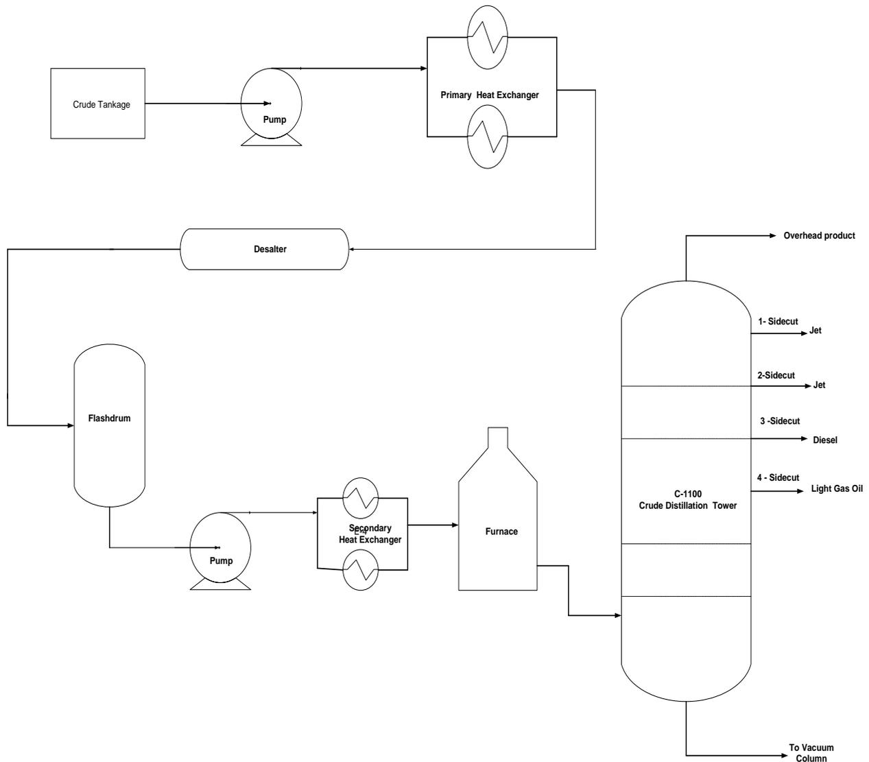
**Figure 4.11. Schematic of diagram of C-1100 Crude unit atmospheric column and upstream process equipment. (CSB 2015).**
