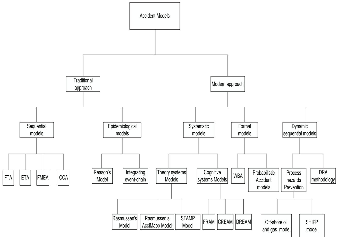
**Figure 3.1. Classification of accident models.**
