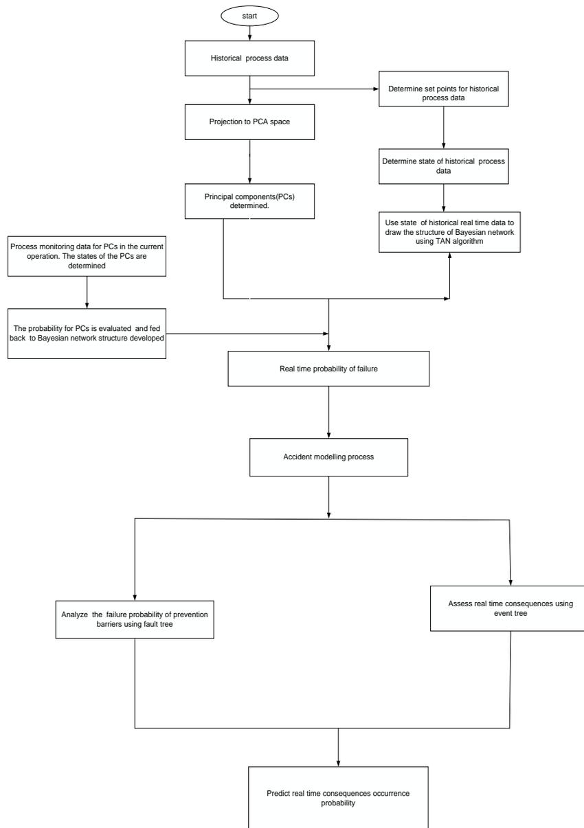
**Figure 6. 3. Proposed accident modelling methodology flowchart.**
