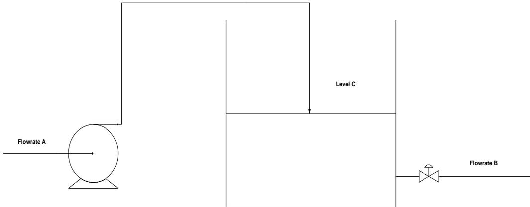
**Figure 7. 1. Simplified flow system of a tank.**
