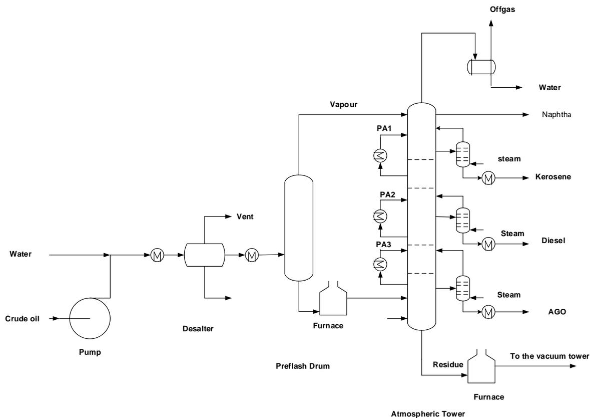
**Figure 6. 5. Process flow diagram of the crude distillation unit. (Al-Mayyahi et al. 2014).**
