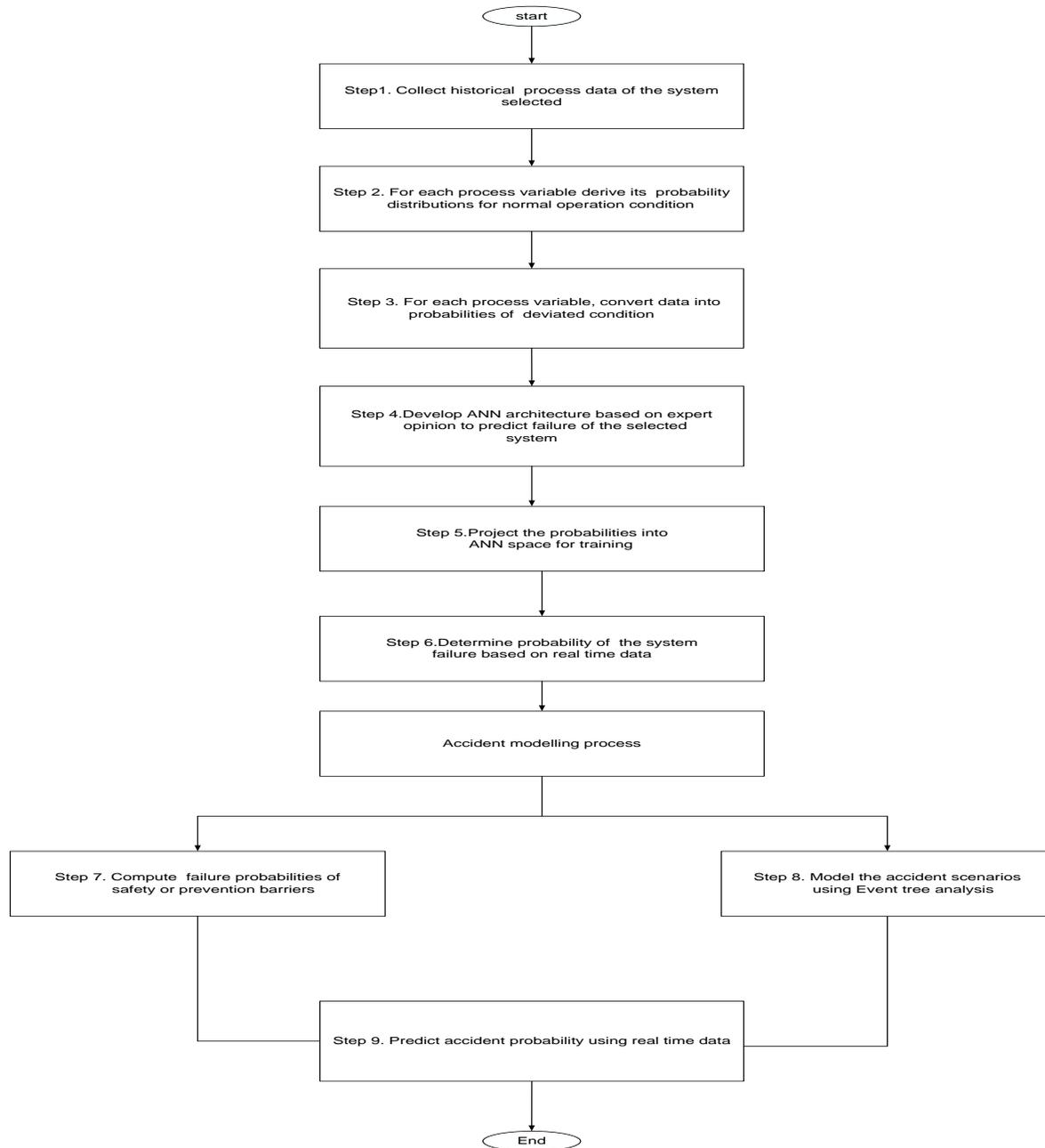
**Figure 7.3. Proposed accident modelling methodology flowchart.**
