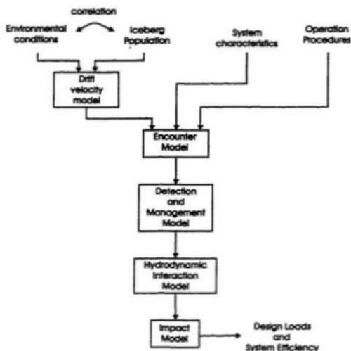
Figure 4.11 Overview of methodology for determining design iceberg impact loads the steps that are required, details will vary depending on the type of system considered.
