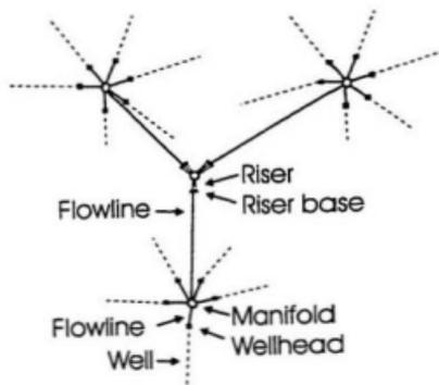
Figure 4.2 Configuration of subsea system
