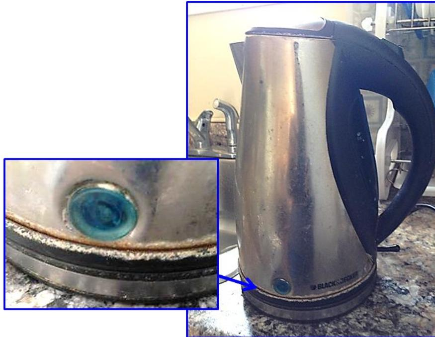
*Figure 16: The electric kettle at one household shows a build-up of off-white, chalky scale from tap water.*
