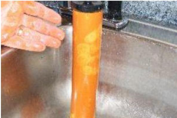
In-house water filter system completely covered in an orange residue after only two months usage - Courtesy Jenny McCarthy.
