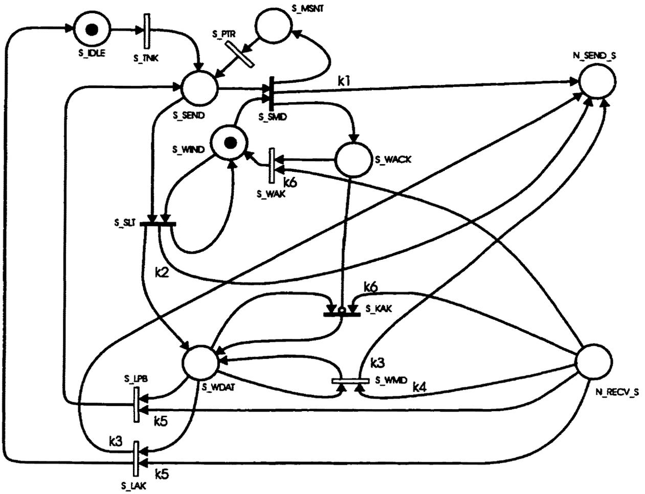
Figure 3.9: TCP Source (SRC) process.
