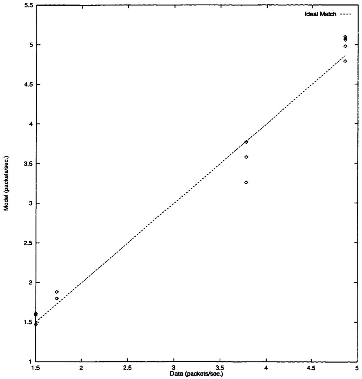
Figure 4.2: Theoretical vs. actual Ethernet packet transmission rates.
