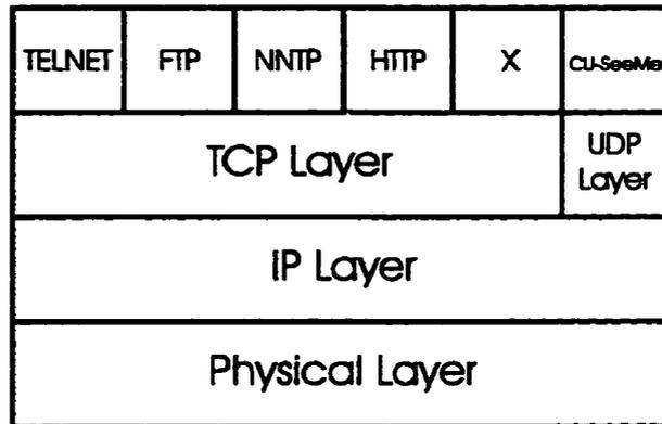
Figure 2.1: TCP/IP protocol stack.
