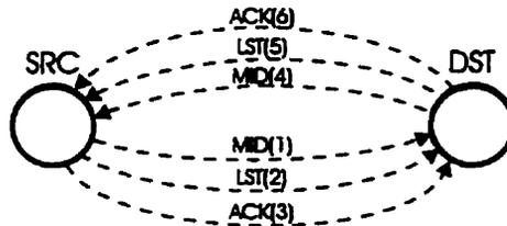
Figure 3.8: Packet flows in model (multiple data types).
