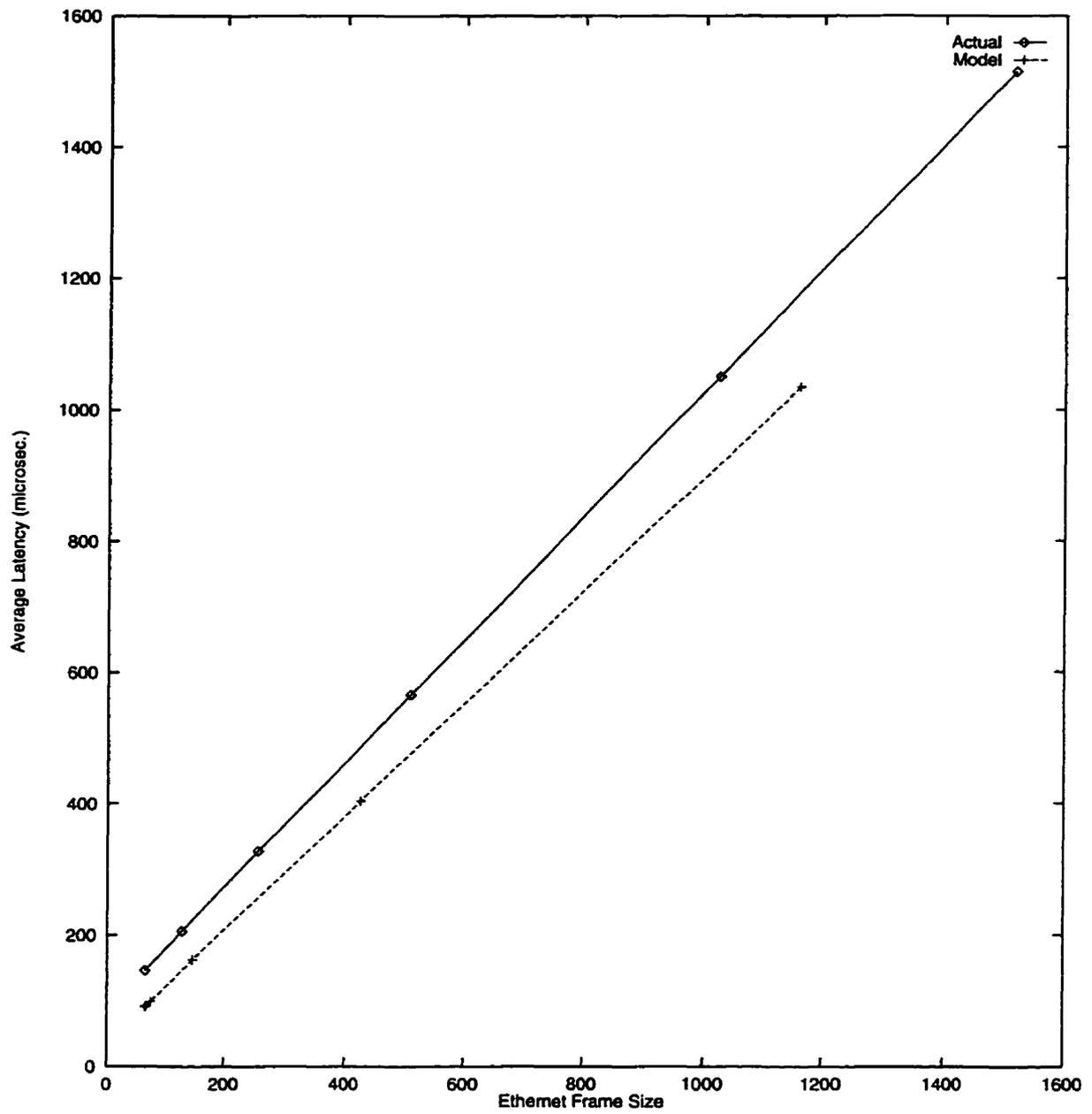
Figure 4.4: Model vs. actual ATM latency.
