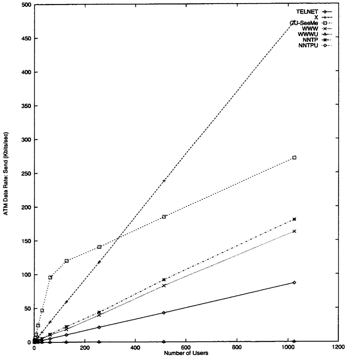
Figure 4.10: Network load by protocol - ATM data rate (send).
