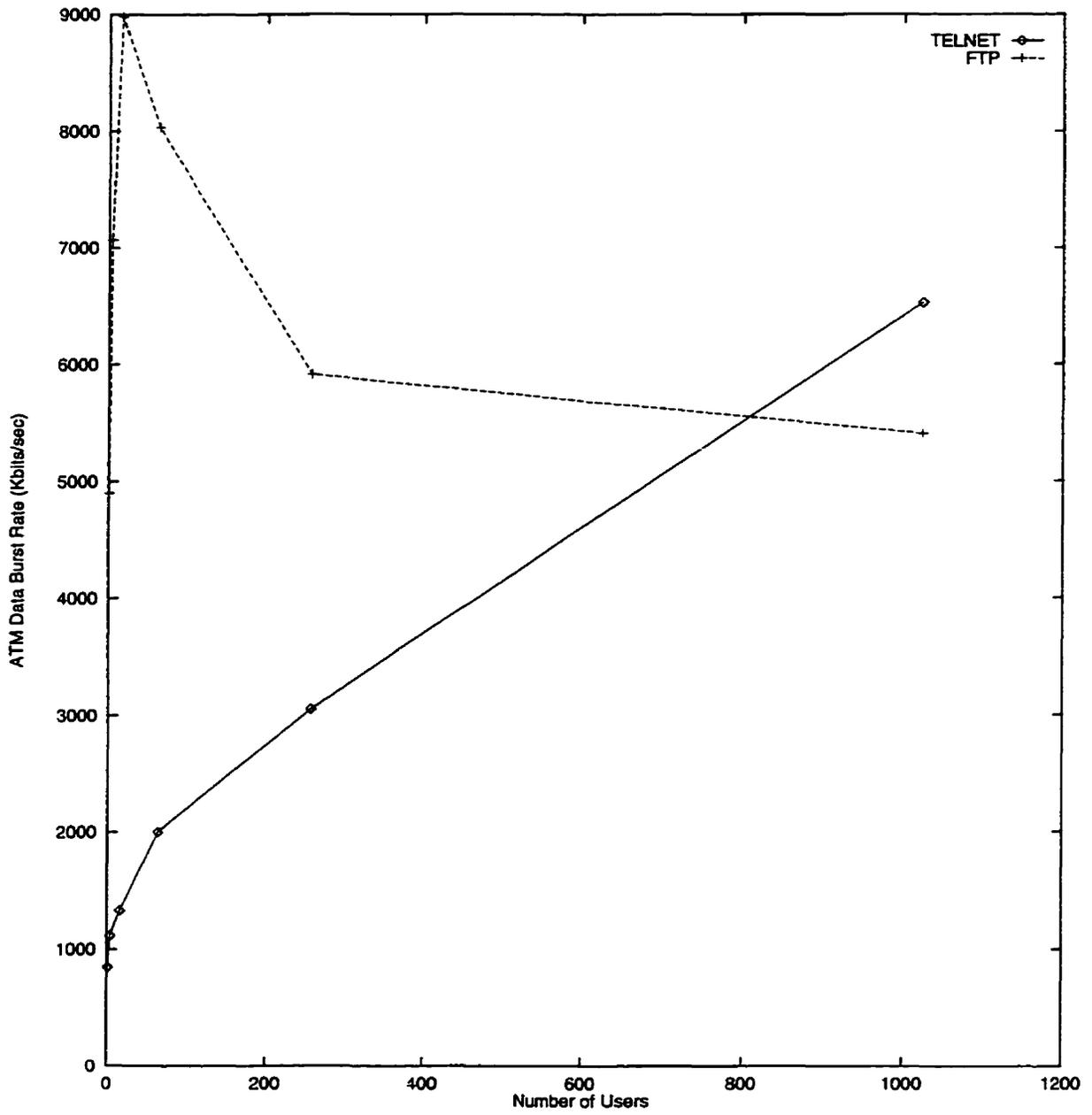
Figure 4.12: Network load by protocol - maximum ATM data rate per user (0.01 ms burst).
