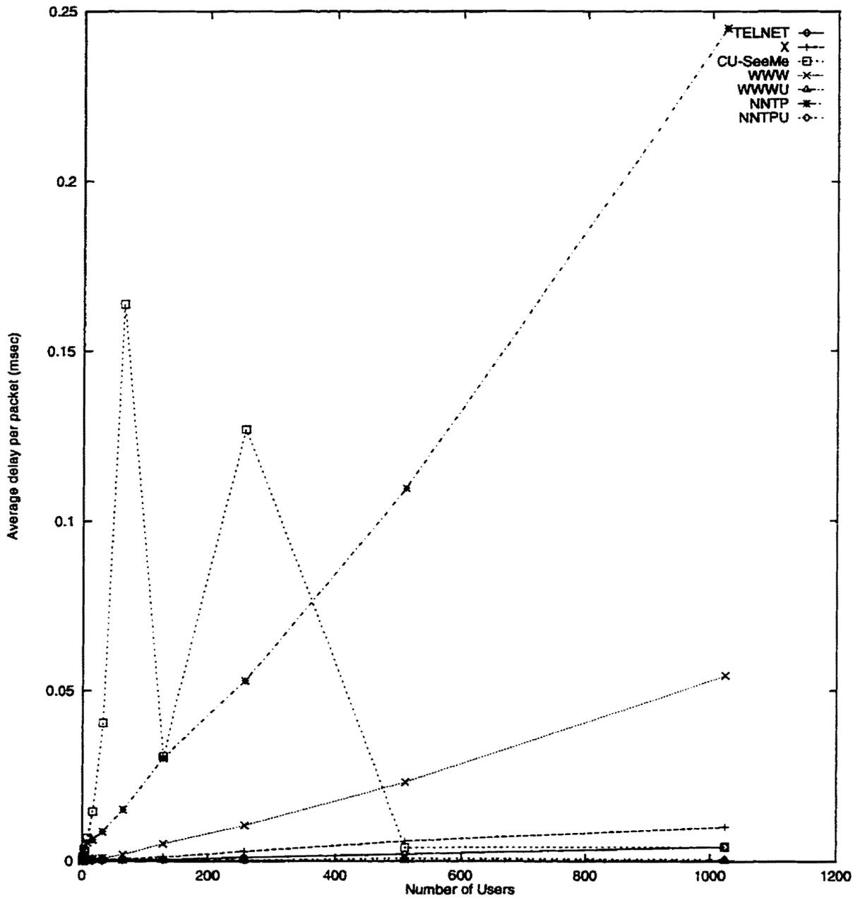
Figure 4.14: Load-induced network delay per packet.
