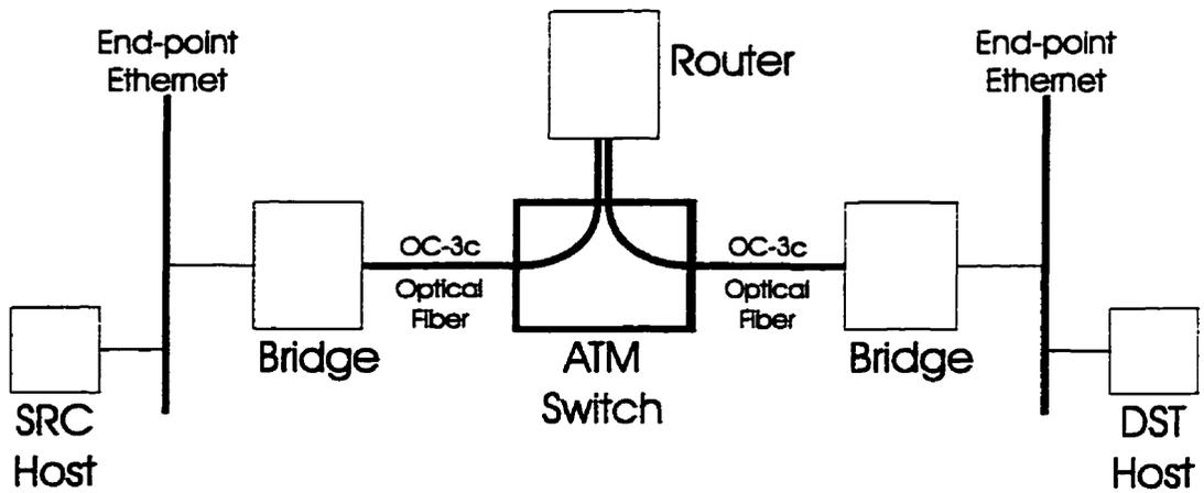
Figure 2.5: Typical data path - different virtual LAN.
