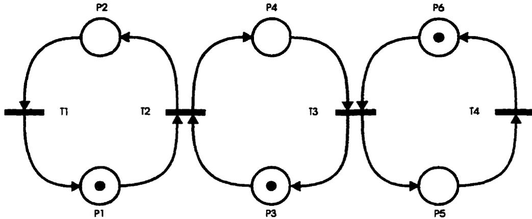
Figure 3.2: Basic Petri net model: producer/consumer bounded-buffer model.
