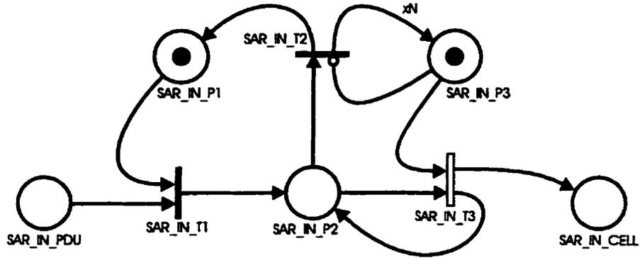
Figure 3.12: AAL (SAR) level - segmentation.
