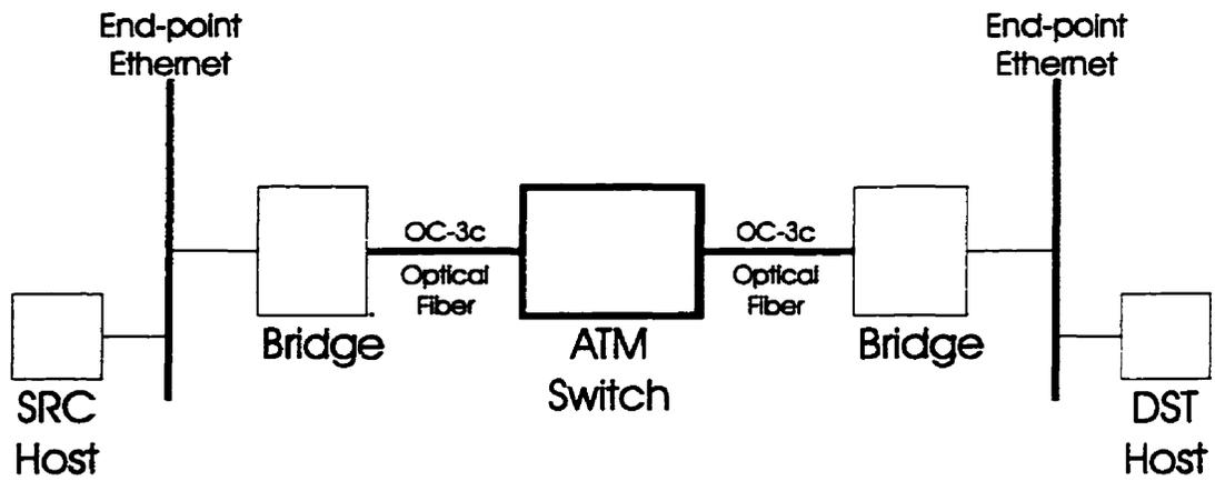
Figure 2.4: Typical data path - same virtual LAN.
