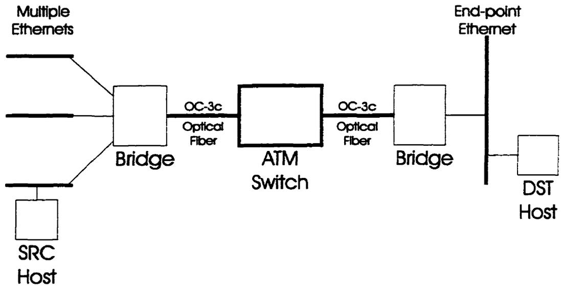
Figure 5.1: LAN Emulation configuration with multiple Ethernets.
