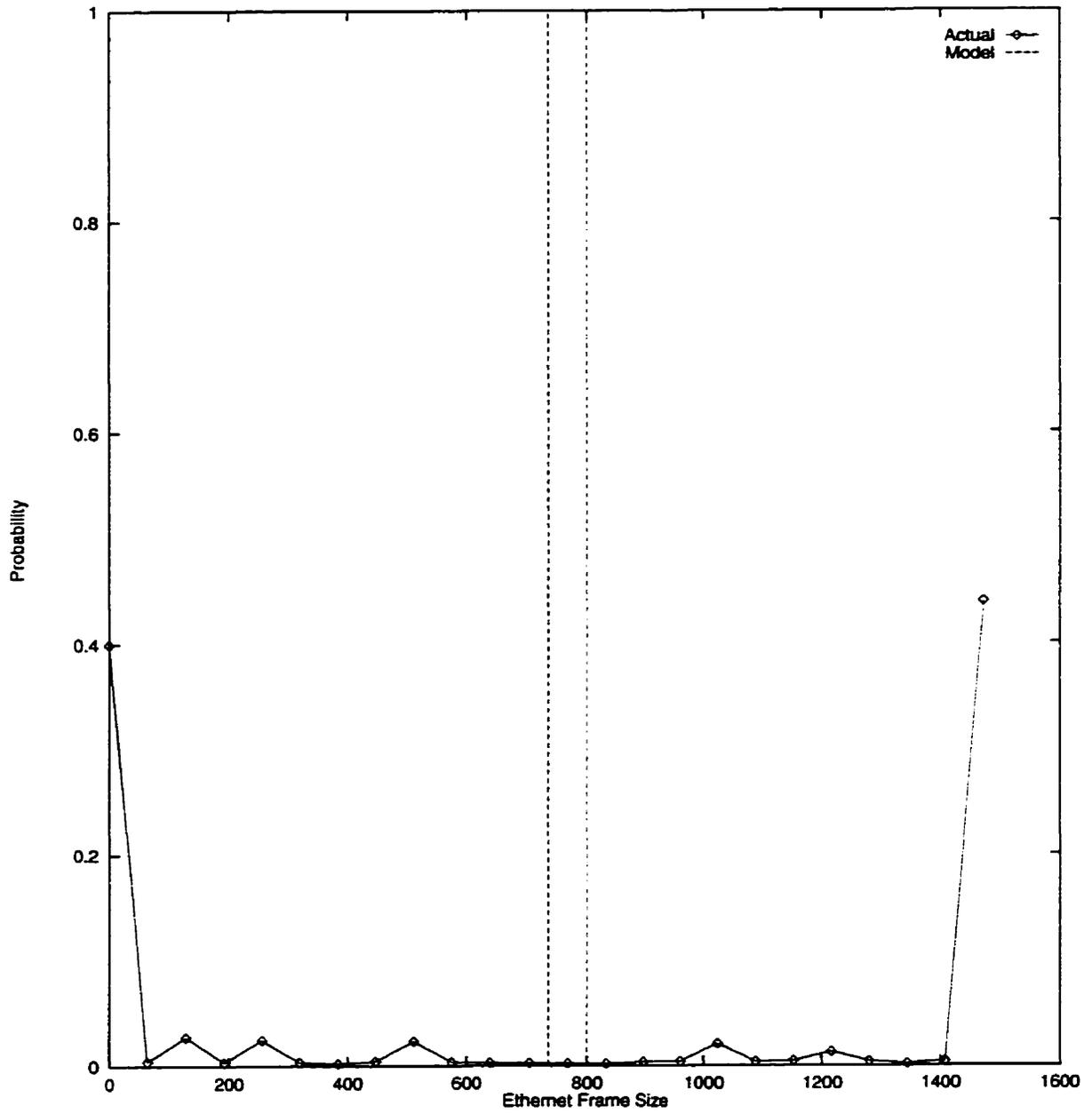
Figure 4.6: Packet size distribution for FTP protocol (single value).
