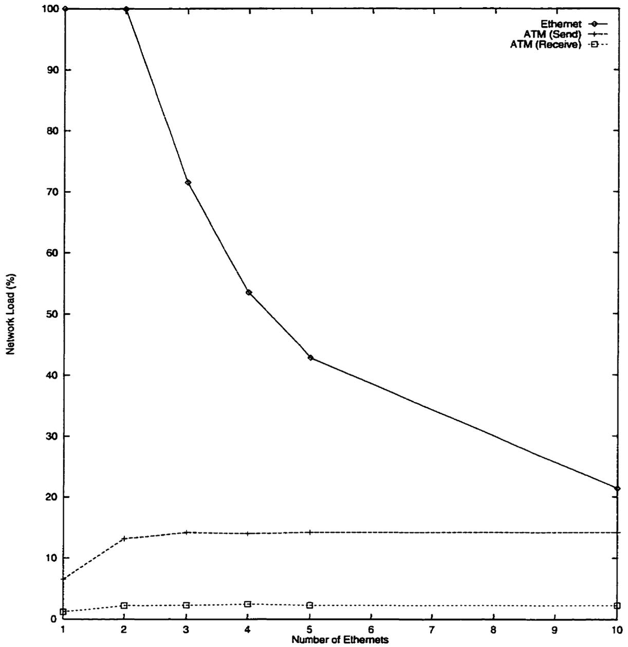
Figure 5.2: Effect on Ethernet and ATM load with multiple Ethernets.
