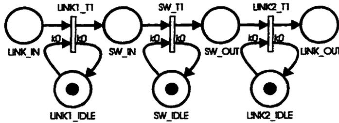
Figure 3.14: ATM switch fabric.
