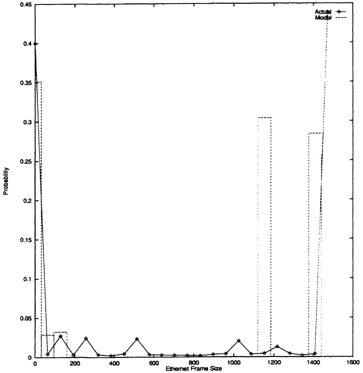
Figure 4.7: Packet size distribution for FTP protocol (multiple packet types).
