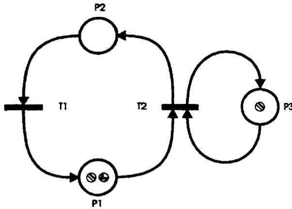
Figure 3.3: Basic Petri net model: coloured version.
