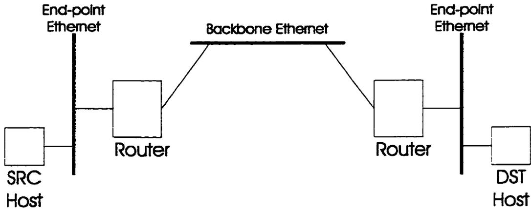
Figure 2.3: Typical data path - old backbone.
