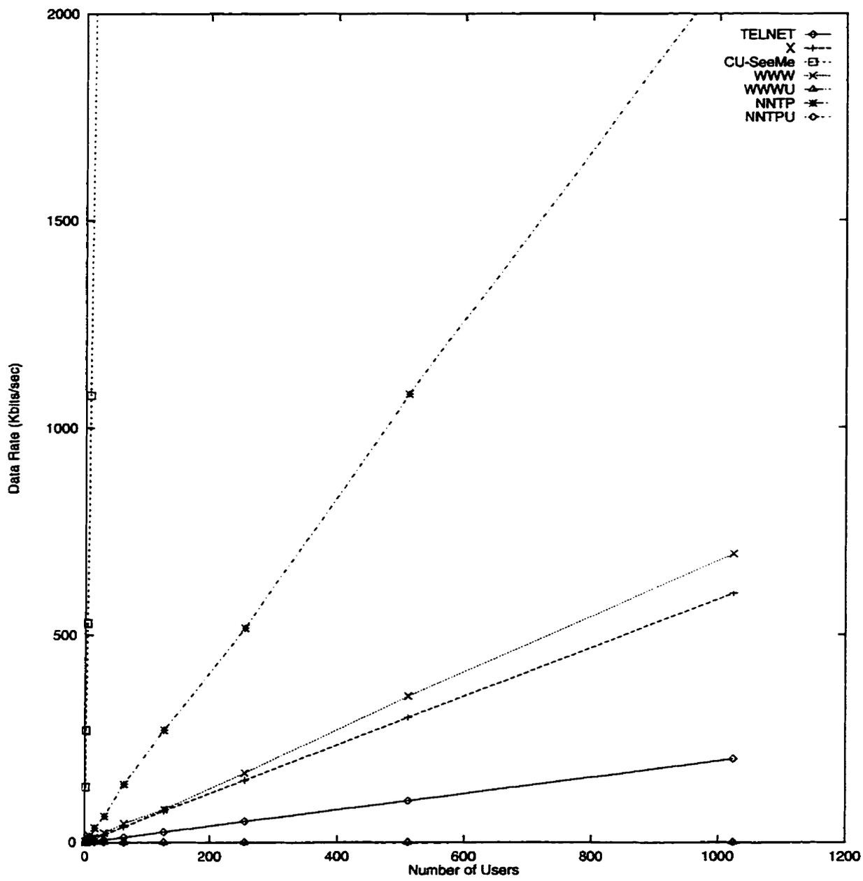
Figure 4.8: Network load by protocol - data rate.
